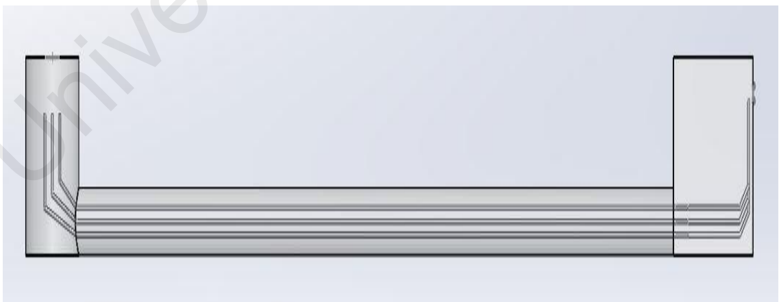
Figure 3.6: Side view of tunnel and cable geometry
