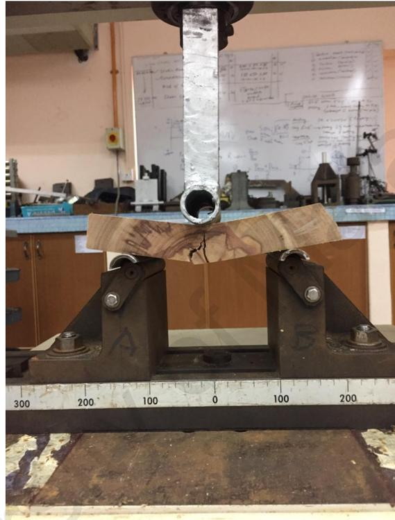
Figure 4.2 Static bending in transverse direction
