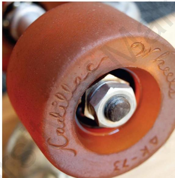
Figure 2.4 The urethane wheel (Snyder, 2015)
