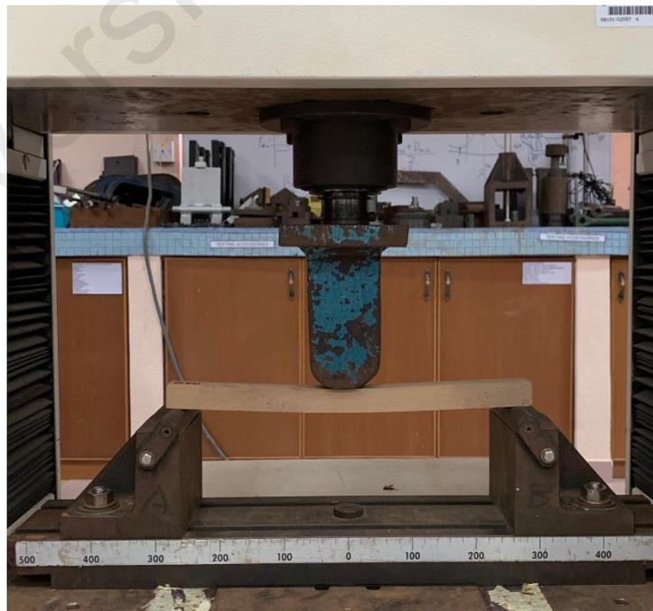
Figure 4.1 Static bending in longitudinal direction
