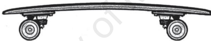
Figure 2.6 Cambered design (Prentiss et al., 2011)
