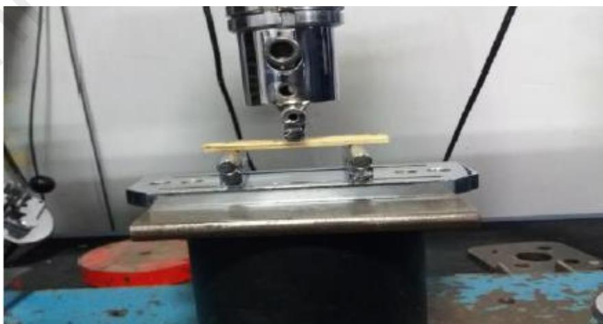
Figure 2.14 The flexural test setup (Munshi & Walame, 2017)
