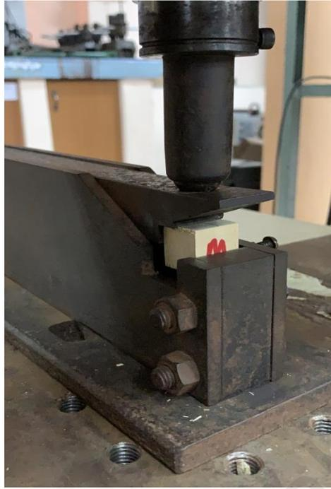
Figure 4.3 Shear test parallel to the grain
