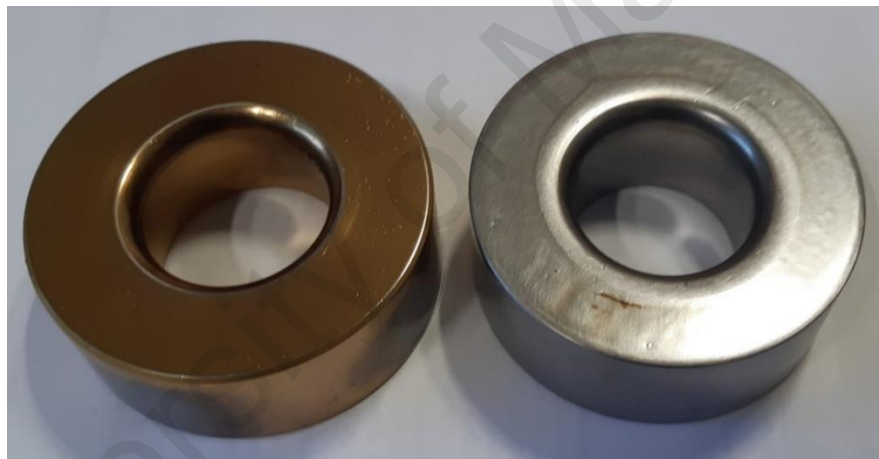
Figure 3.3: TiN coated die (right) and SKD-11 tool steel uncoated die (left)
