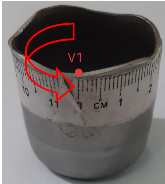
Figure 4.10: Measurement of thickness distribution along the circumference direction
