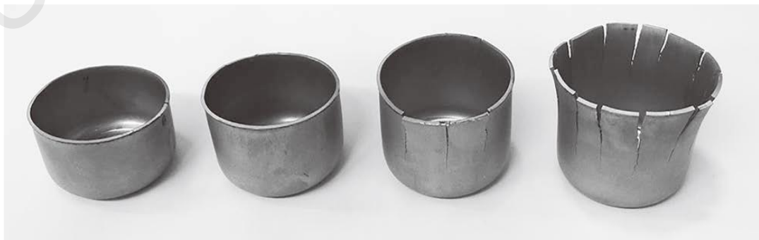
Figure 2.12: Stainless steel 301 deep drawn cups at drawing ratios 1.8, 1.9, 2.0 and 2.12 (Papula et al., 2015)
