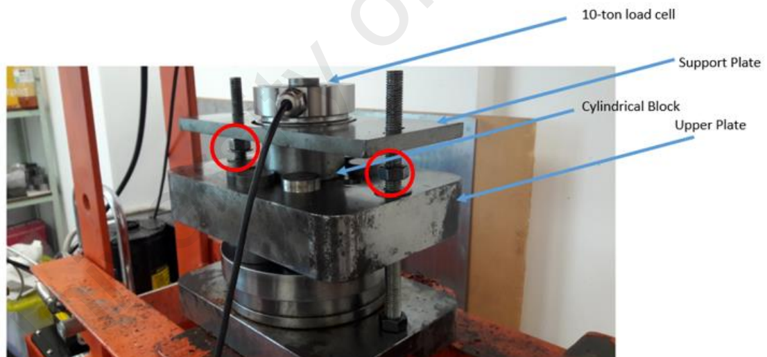
Figure 3.7: Setup for generating and measure the target BHF
