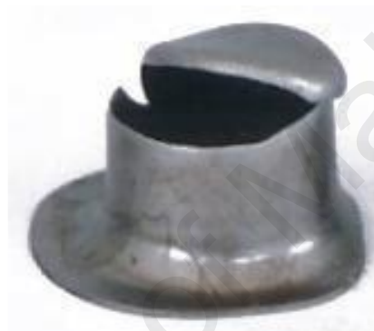
Figure 2.3: Fracture in deep drawing (Swapna et al., 2018)
