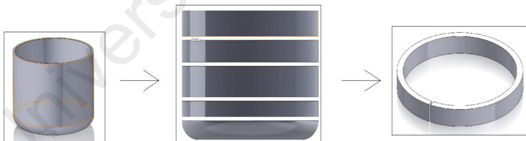
Figure 3.9: Ring slitting method
