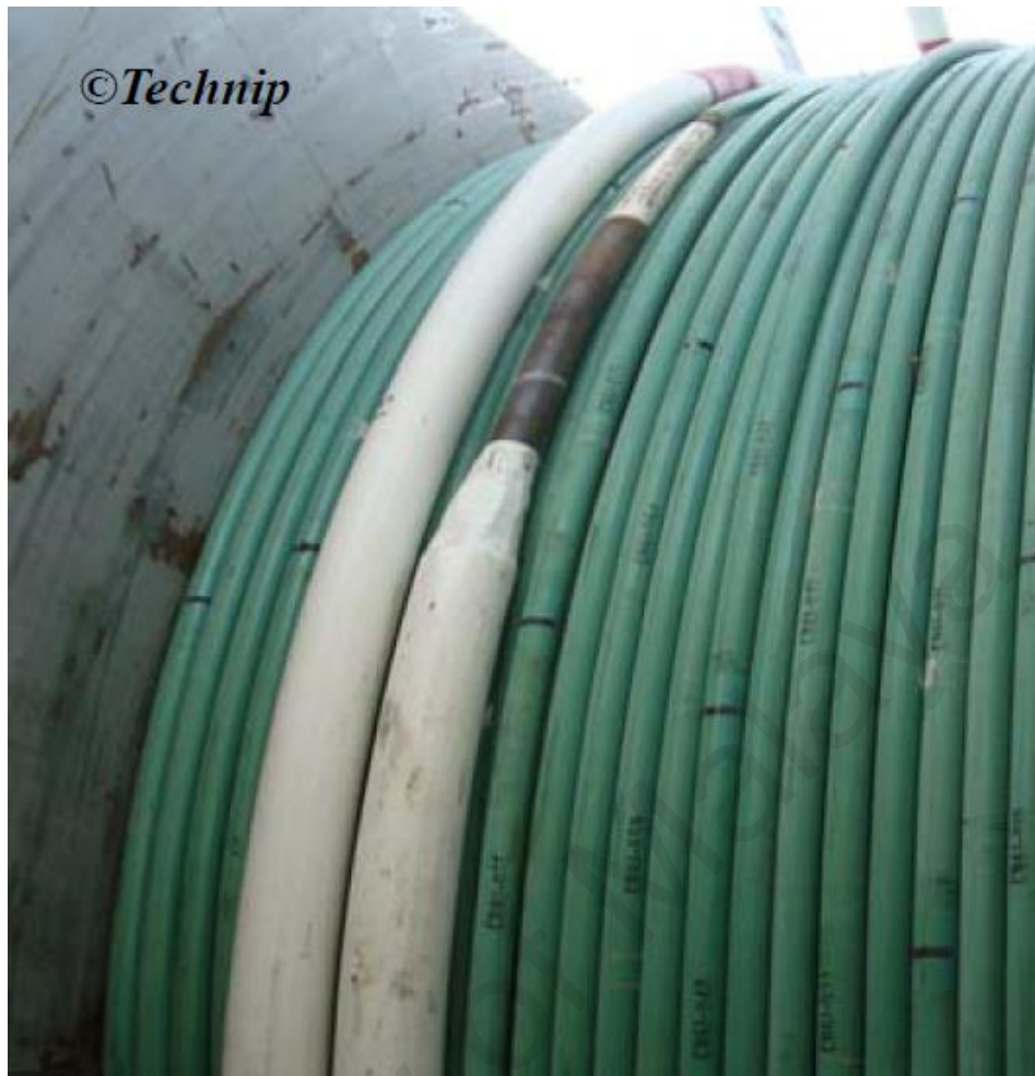
Figure 2.9: Transition Joint on Reel Drum Courtesy of Technip
