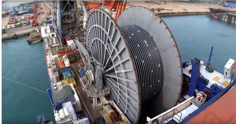
Figure 2.4: Pipeline Reeling Operation on LV NO105 (McDermott Legacy, 2014)
