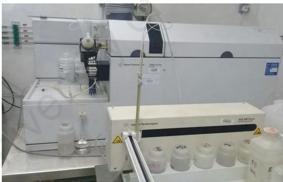
**Figure 3.1: Inductively Coupled Plasma Mass Spectrometer (ICP-MS, Agilent 7500ce).**
