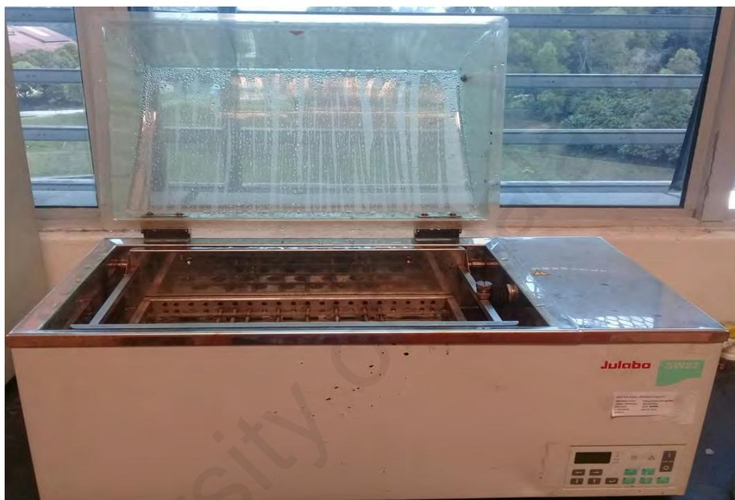
**Figure 3.4: Shaking Incubator (Julabo SW22).**
