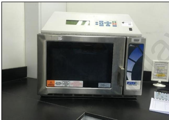
**Figure 3.2: The scientific microwave processor (Labpulse 2850), used in the experiment for heat induced antigen retrieval**
