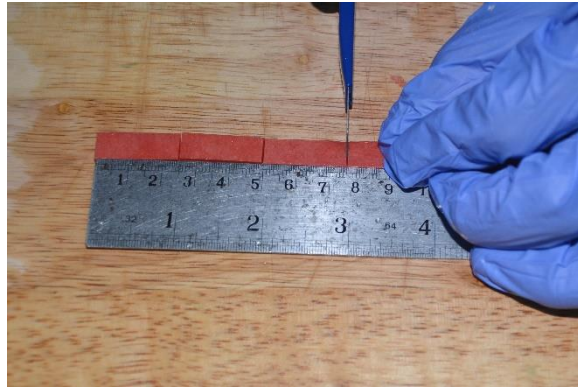
Figure 3.7: Cutting specimens of chewing gum (25-mm-length)
