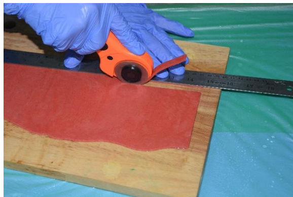
Figure 3.6: Roller cutter used to cut strip of chewing gum (10-mm-width)
