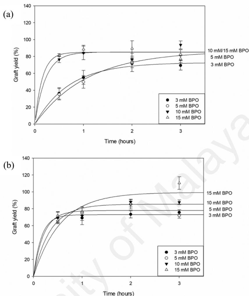
**Figure 4.10:** Graft yield as a function of incubation time, for (A) 70 °C and (B) 90 °C incubation temperature. Initial BPO concentrations at 3-, 5-, 10- and 15 mM for both temperatures. Initial mcl-PHA and GDD concentrations were 50 g L<sup>-1</sup> and 0.14 M respectively in 4 ml of acetone
