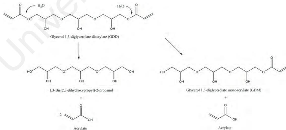
**Figure 4.6:** Thermal degradation of GDD to produce acrylate monomers *via* hydrolysis
