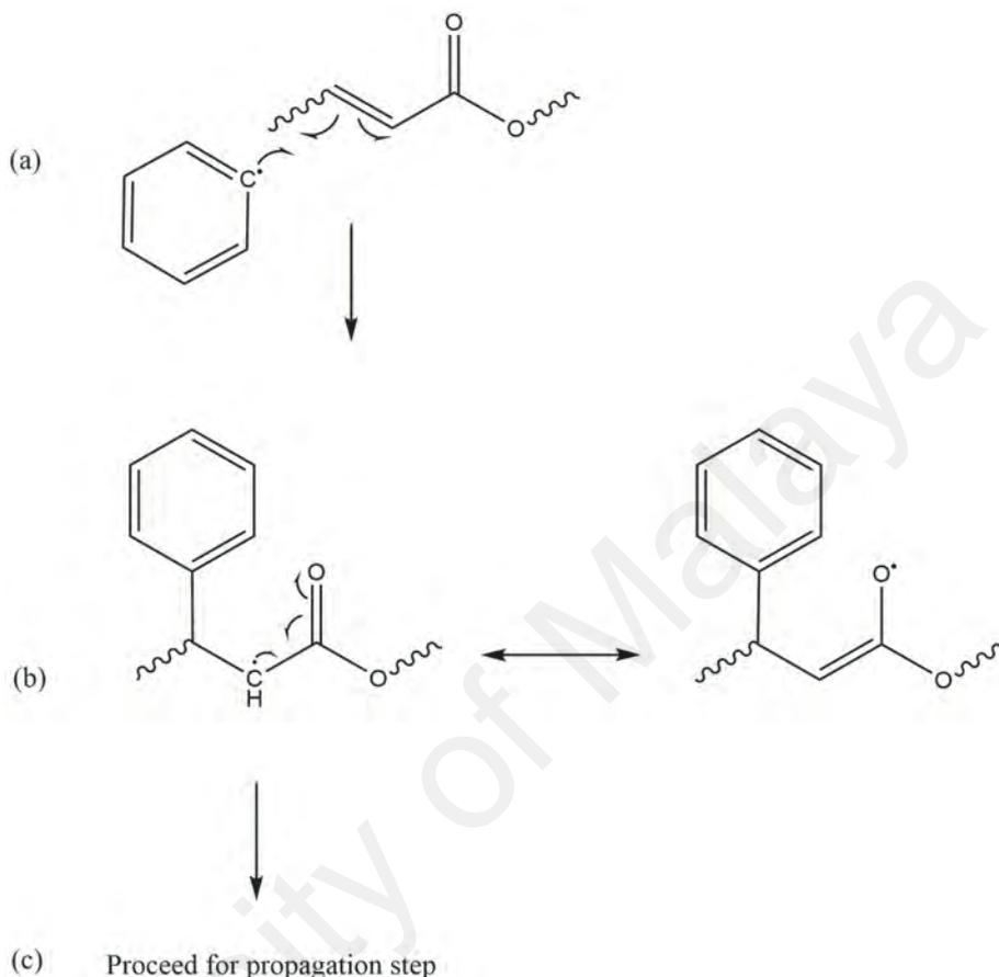
**Figure 4.8:** The allylic resonance involved after radical intervention on the reaction species, (a) benzene radical attacked the species with alkenyl group, (b) the allylic resonance shows the movement of the unpaired electron along the bonds, and (c) entering propagation step
