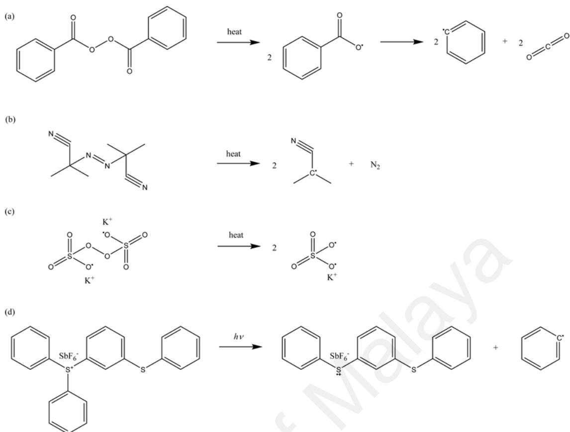
**Figure 2.5:** Thermal decompositions of (a) benzoyl peroxide, (b) AIBN, and (c) potassium persulfate, meanwhile irradiation-induced decomposition of (d) triaryl sulfonium salt
