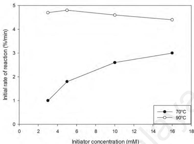
**Figure 4.12:** Initial rate of reaction for GDD grafting of mcl-PHA as a function of starting initiator concentration. The initial mcl-PHA and GDD concentrations were 50 g L<sup>-1</sup> and 0.14 M respectively in 4 ml of acetone
