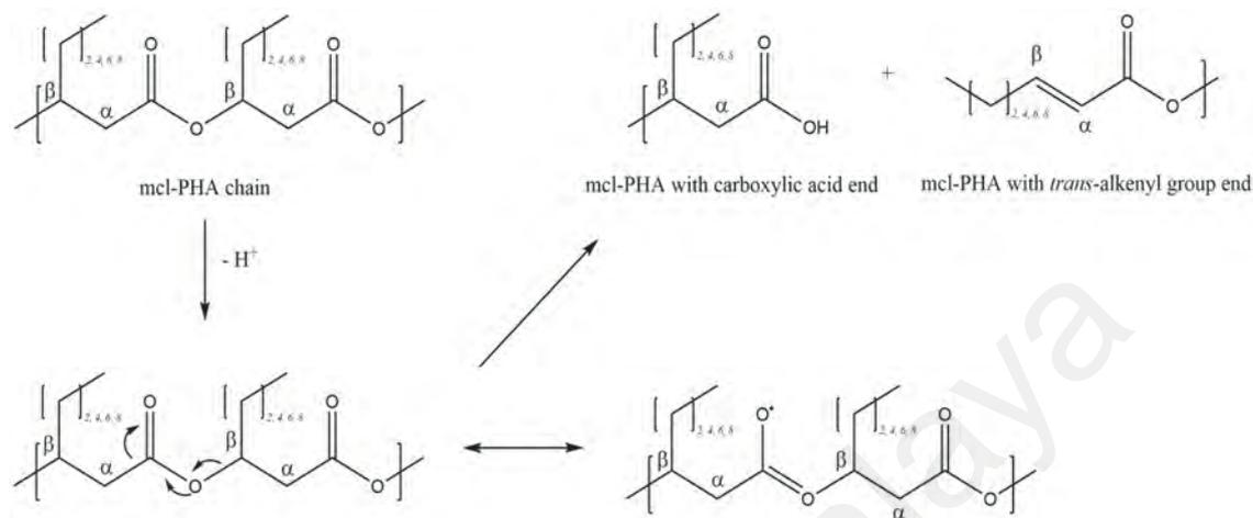
**Figure 4.5:** Possible routes of mcl-PHA degradation that contribute to alkenyl end group able to participate in grafting reaction *via* proton abstraction
