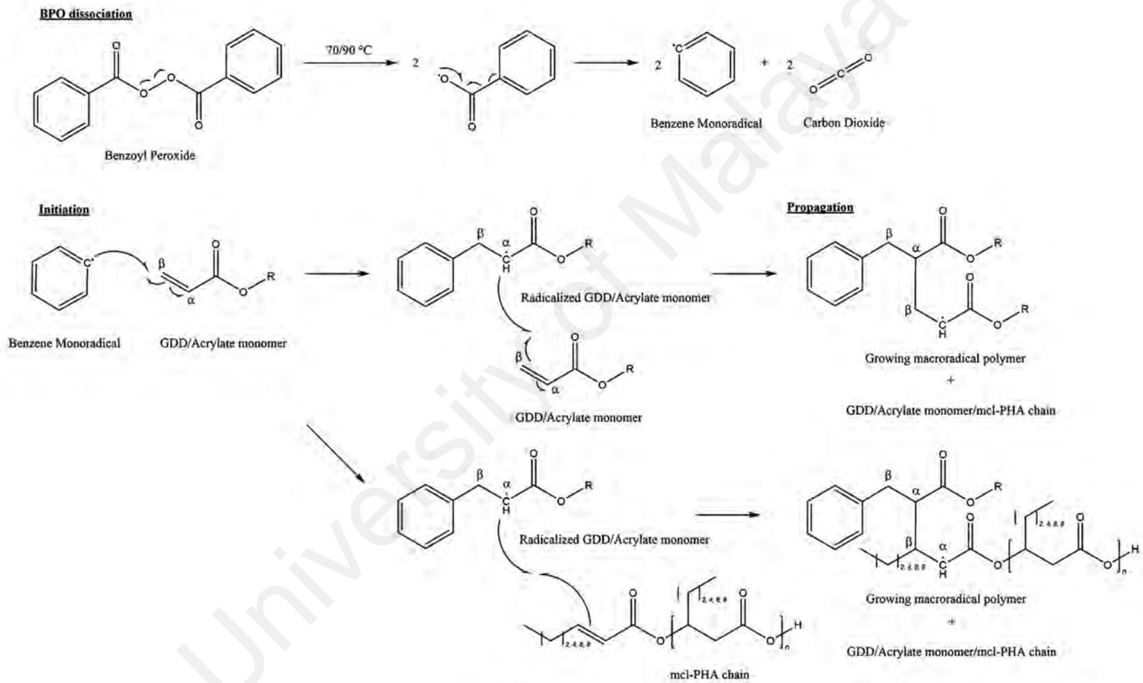
**Figure 4.7:** Proposed mechanism for graft copolymerization involving GDD and mcl-PHA
