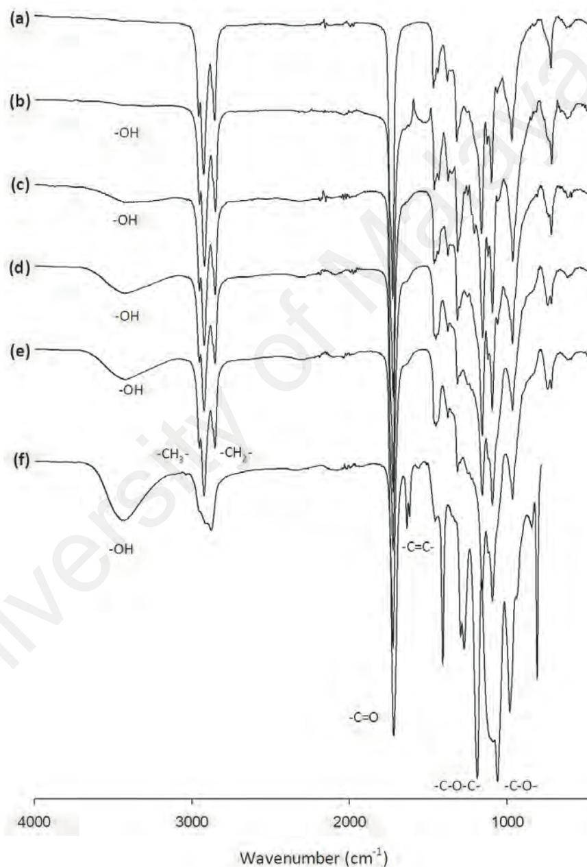
**Figure 4.1:** FTIR spectra of grafted materials obtained from reaction mixture at 70 °C. (a) mcl-PHA; (b) PHA-g-GDD with 3 mM BPO; (c) PHA-g-GDD with 5 mM BPO; (d) PHA-g-GDD with 10 mM BPO; (e) PHA-g-GDD with 15 mM BPO; and (f) GDD monomer
