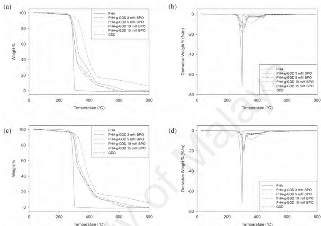
**Figure 4.9:** TGA analysis for PHA, PHA-g-GDD and GDD samples for different initiator concentrations, (a) & (c) weight percentage curves, and (b) & (d) derivative weight percentage curves, while (a) and (b) represent samples incubated at 70 °C and (c) and (d) at 90 °C
