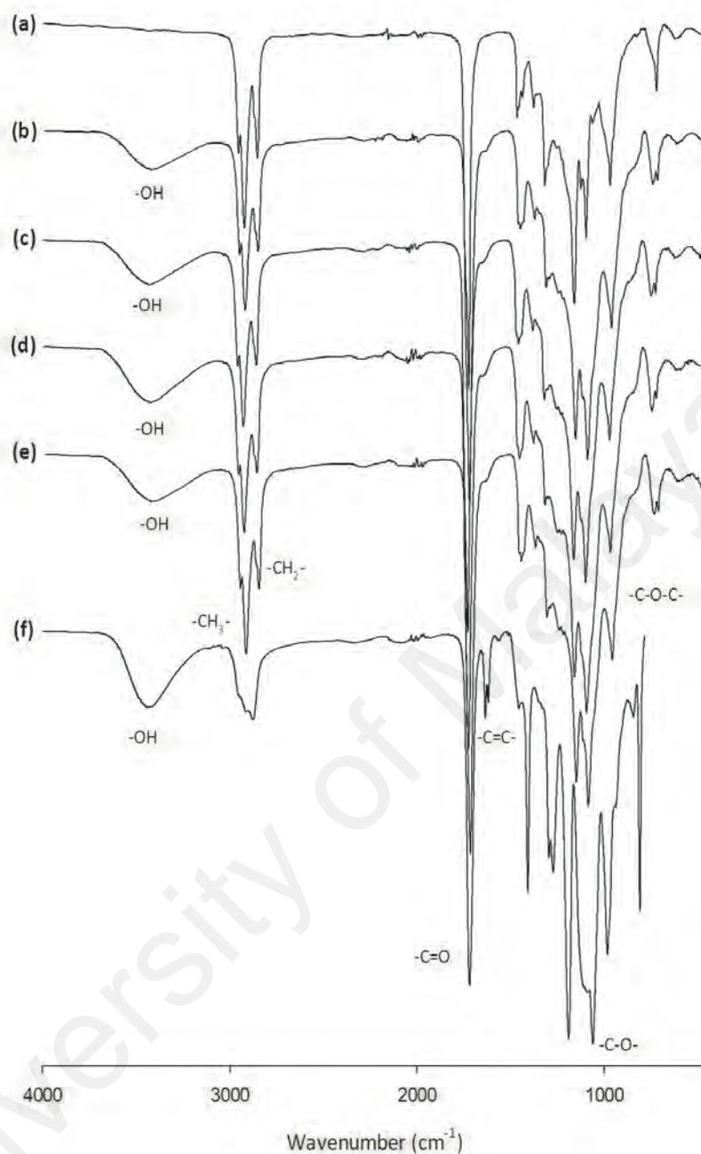
**Figure 4.2:** FTIR spectra of grafted materials obtained from reaction mixture at 90 °C. (a) mcl-PHA; (b) PHA-g-GDD with 3 mM BPO; (c) PHA-g-GDD with 5 mM BPO; (d) PHA-g-GDD with 10 mM BPO; (e) PHA-g-GDD with 15 mM BPO; and (f) GDD monomer
