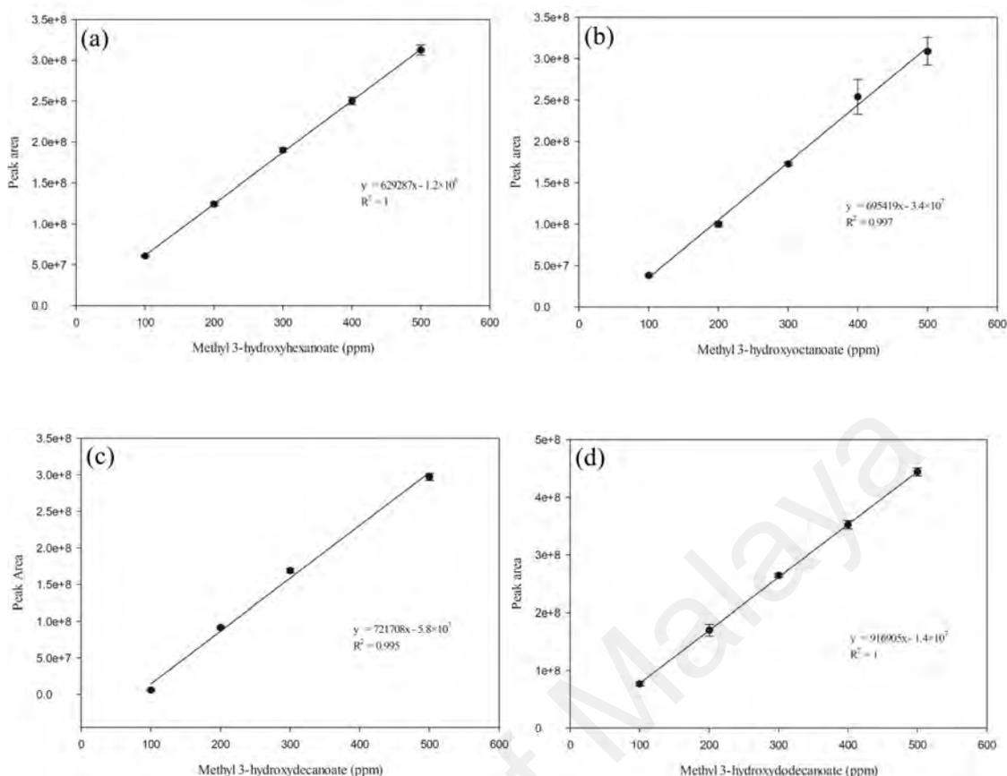
**Figure 3.1:** GC calibration plot for standard monomer concentration (a) Methyl 3-hydroxyhexanoate; (b) Methyl 3-hydroxyoctanoate; (c) Methyl 3-hydroxydecanoate; and (d) Methyl 3-hydroxydodecanoate
