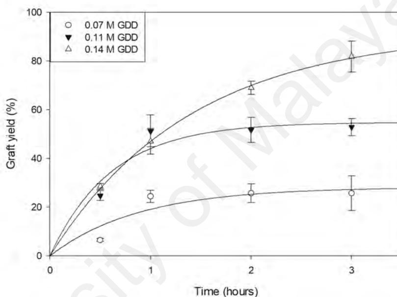
**Figure 4.11:** Graft yield as a function of incubation time for different GDD concentrations at 70 °C incubation. Initial mcl-PHA and BPO concentrations were 50 g L<sup>-1</sup> and 10 mM respectively in 4 ml of acetone
