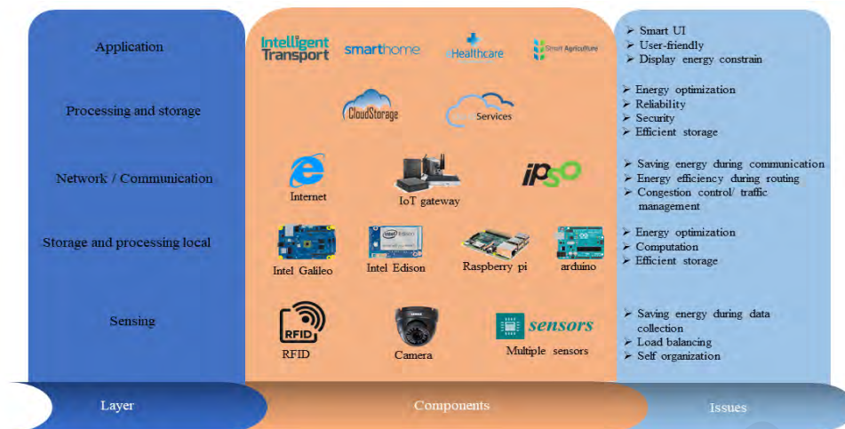
Figure 2.4: IoT Layered architecture for energy consumptions 2
