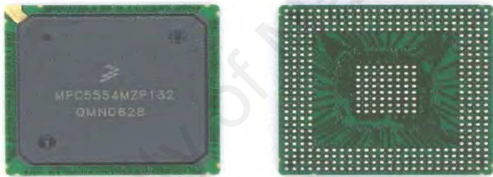
Figure 2.1: Typical PBGA package
