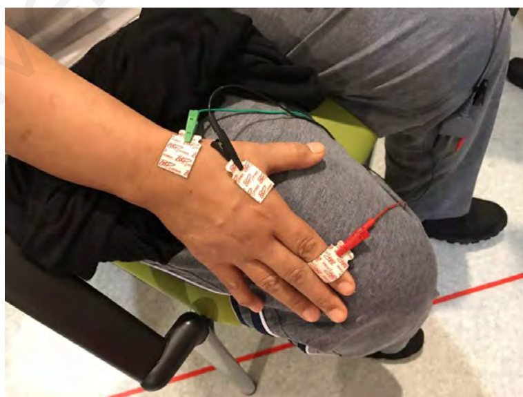
Figure 3.4: An image of the placement of electrodes on the hand muscles.
