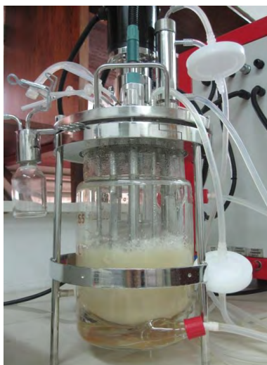
Figure 3.2: Two litre stirred tank bioreactor containing of 10% (v/v) of liquid inoculum in optimised medium consisting of 2% brown sugar, 1% baker's yeast, 1% spent grain extract, 0.5% Tween 80, 0.05% MgSO 4 , 0.05% KH 2 HPO 4 and 0.05% K 2 HPO 4 .
