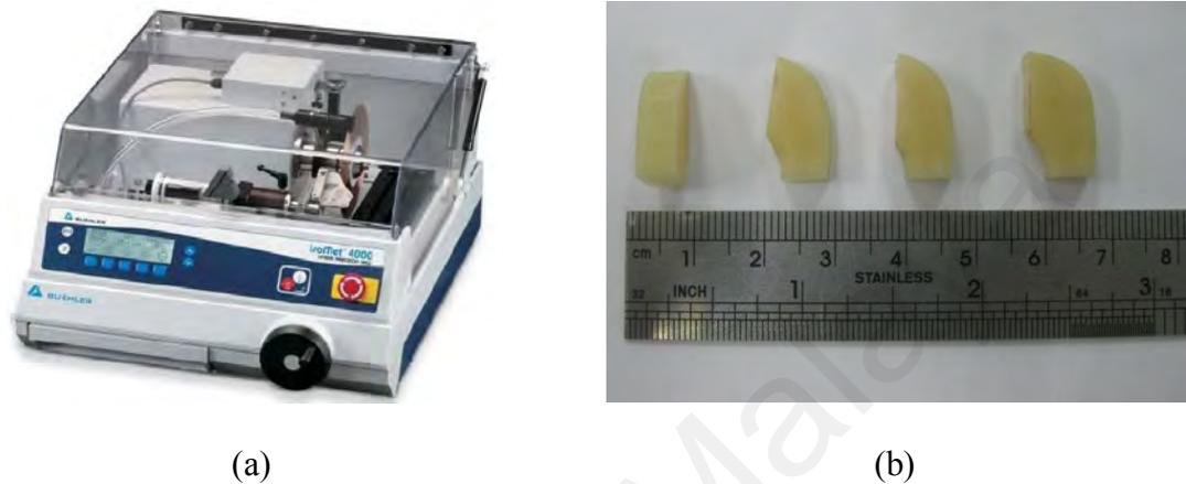
Figure 3.2: The precision saw (a) used to cut the test samples (b).
