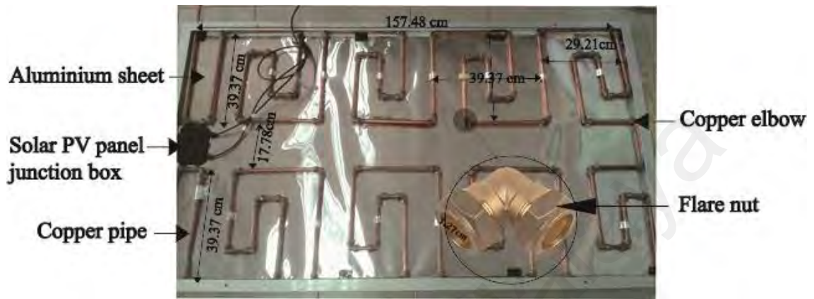
Figure 3.9: Double serpentine flow channel attached to PV rear side
