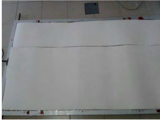
Figure 3.12: Ceramic fiber insulation cover on PV/T rear side
