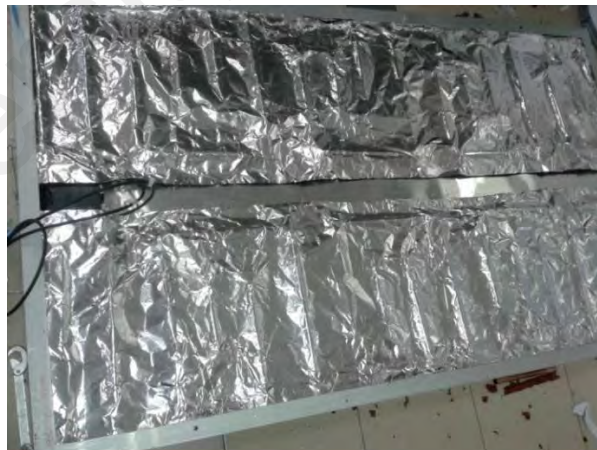
Figure 3.11: Aluminum foil cover on the thermal collector
