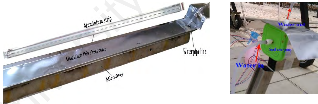
Figure 3.17: Sweeping microfiber and water flow pipeline
