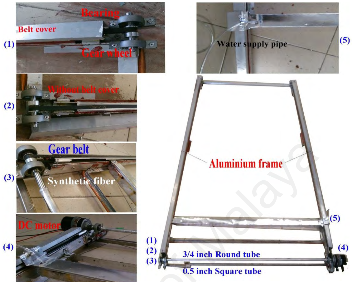
Figure 3.18: Complete self-cleaning system
