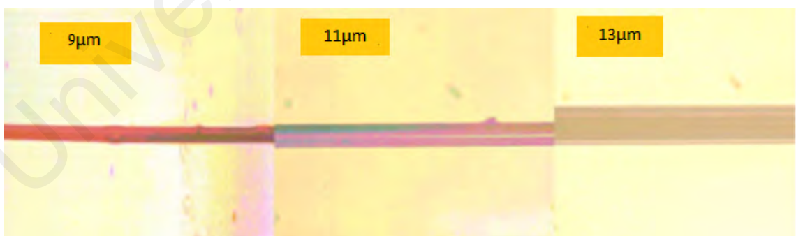
Figure 5.3: PMMA microfibers with three different waist diameters (a) 9 \mu\text{m} (b) 11 \mu\text{m} and (c) 13 \mu\text{m}
