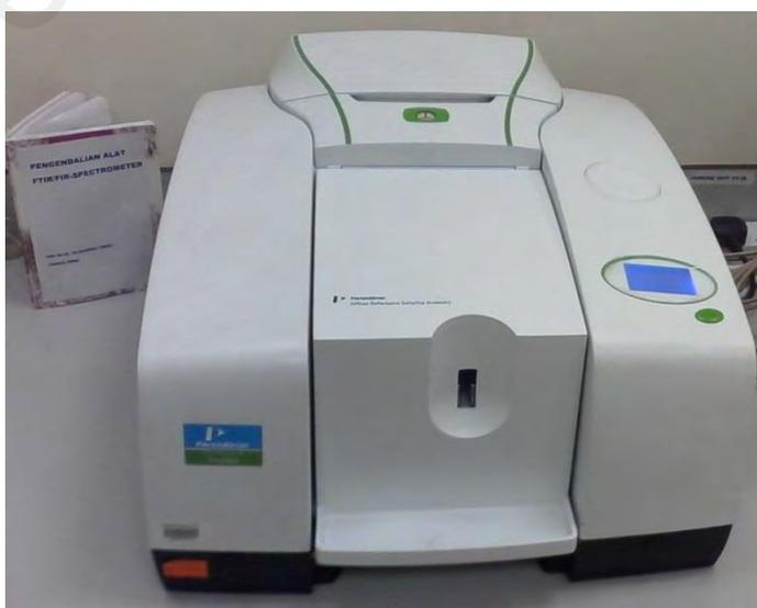
**Figure 3.6: Perkin Elmer Frontier FTIR spectrometer**
