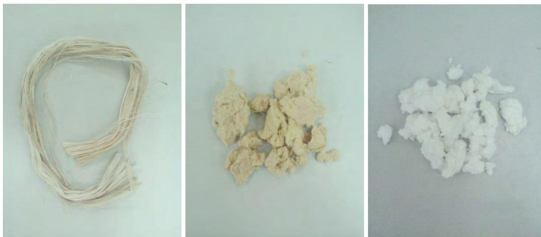
**Figure 3.2: Photographs of (a) kenaf fiber, (b) fiber after alkali treatment and (c) lignin-free cellulose**
