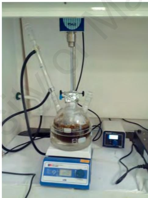
**Figure 3.1: Alkali treatment and bleaching process**
