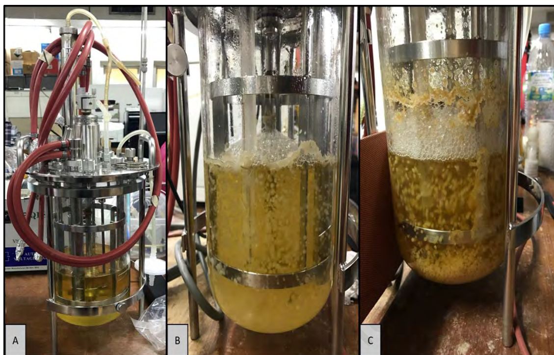
Figure 4.13: Process of large-scale biomass production of G. lucidum in Bioreactor 2-L (Sartorius Biostat A plus). Image A shows Bioreactor 2-L (Sartorius Biostat A plus) without inoculation. Image B shows Bioreactor 2-L (Sartorius Biostat A plus) inoculated with G. lucidum . (Day 3) [Working volume = 1.5-L] and image C shows Bioreactor 2-L (Sartorius Biostat A plus) inoculated with G. lucidum . (Day 10) [Working volume = 1.5-L]
