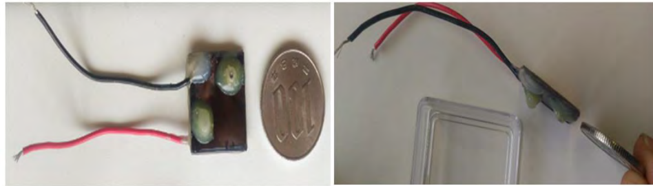
Figure 7.15. Finished single TEC device with cross section area 2 \times 2 \text{ cm}^2 and 0.3 mm electrode separation
