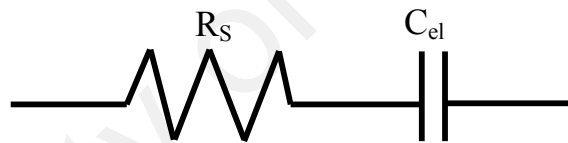
Figure 2.20. Equivalent circuit of double layer formation
