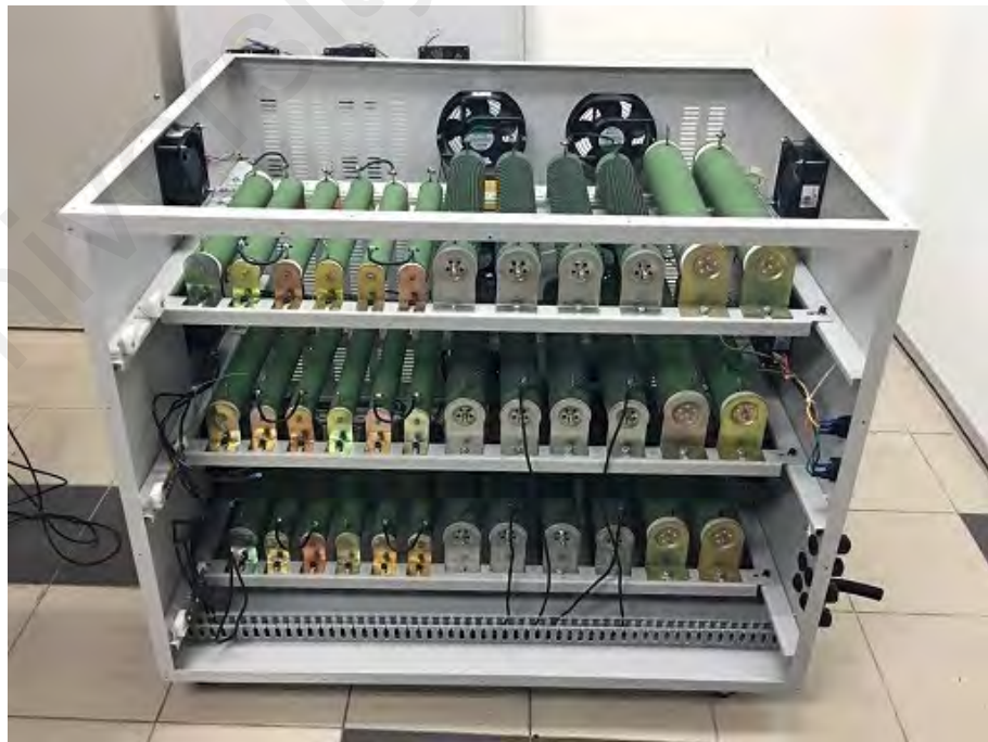
Figure 5.6: The load bank which contains all the resistive loads.
