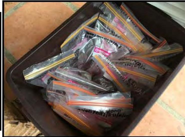
**Figure 3.12:** The collected soil samples.
