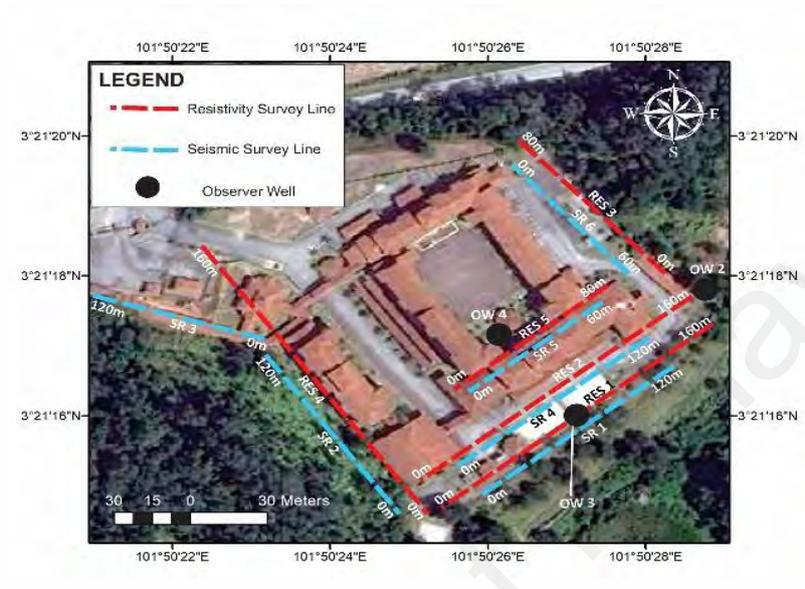
**Figure 3.5:** A plan view of the school compound and preliminary areas of investigation using geophysical techniques (modified from Google Maps, 2018).
