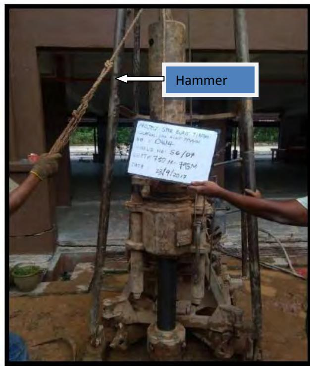
**Figure 3.10:** The image showing a standard penetration test.
