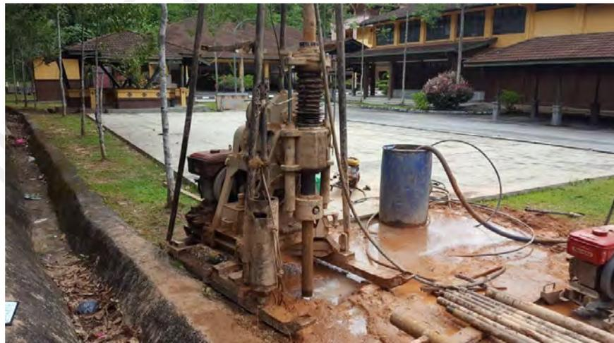
**Figure 3.9:** The image showing the skid drilling machine.
