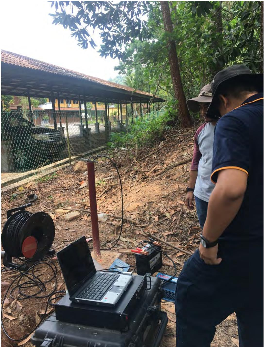
**Figure 3.14:** The Colloidal Borescope System instrument.
