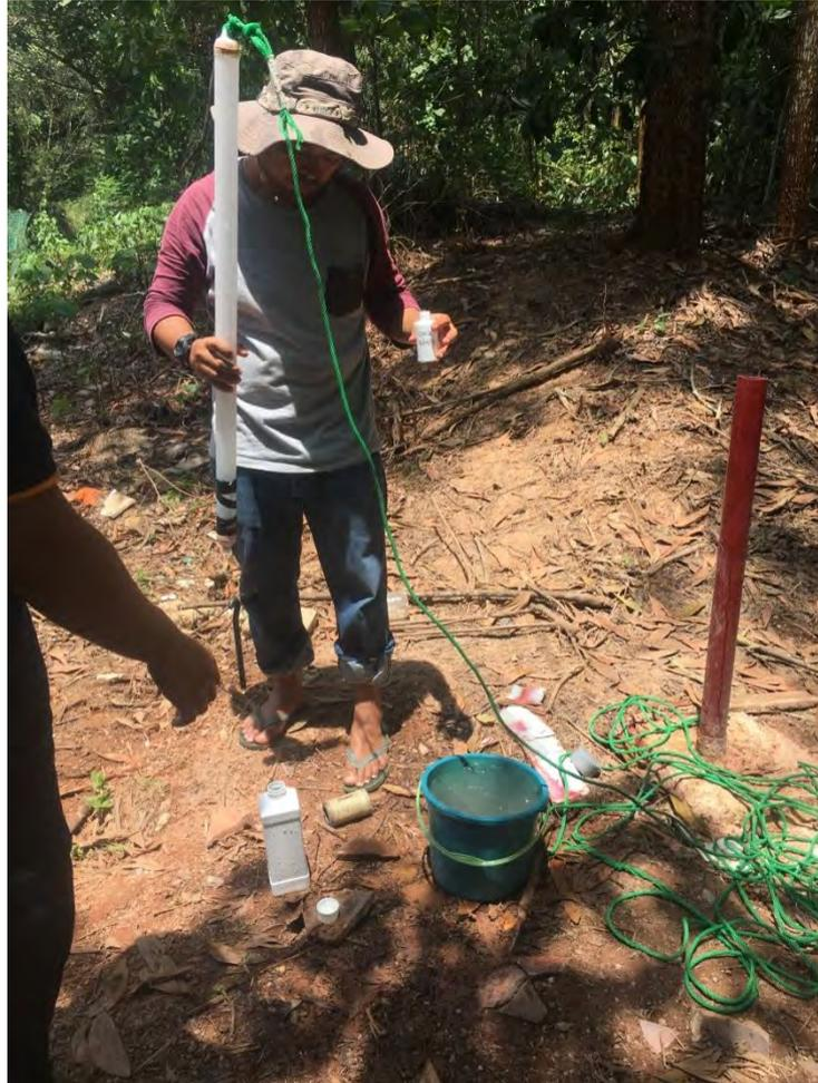
**Figure 3.16:** Collection of water samples by a manual bailer.
