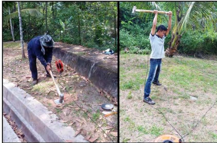
**Figure 3.8:** Creating seismic energy by vertically striking a solid metal plate with a sledgehammer.
