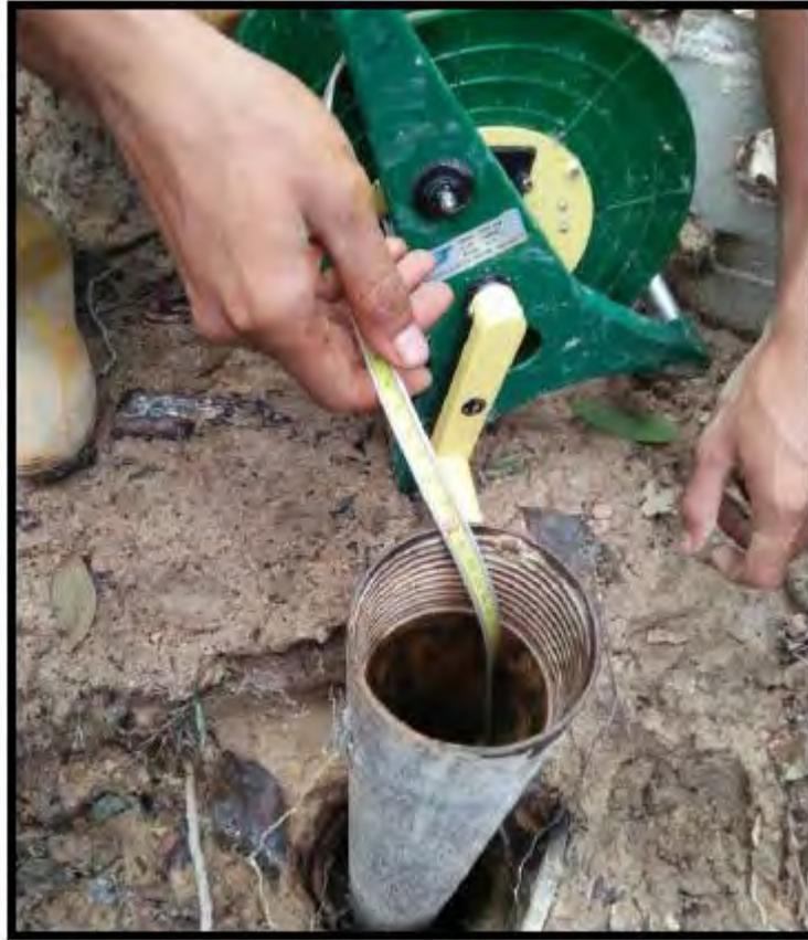
**Figure 3.15:** Water level monitoring using a dipmeter.
