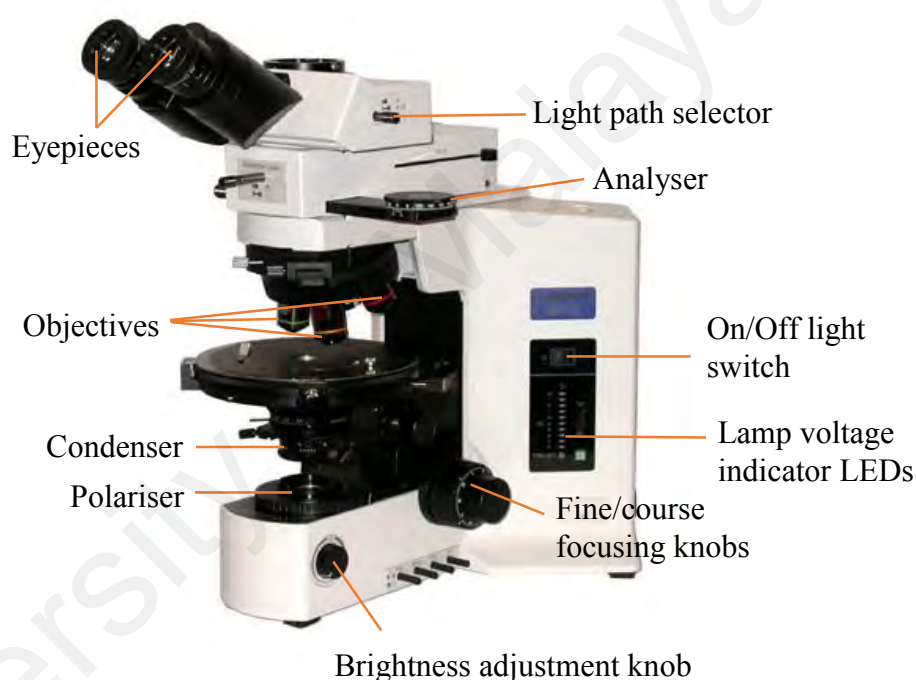
Figure 3.2: A schematic setup of an optical polarising microscope. Redrawn from (Robinson & Davidson, 2016).
