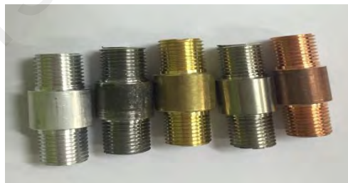
Figure 3.9: Coupons of different materials on heat exchanger surfaces.
