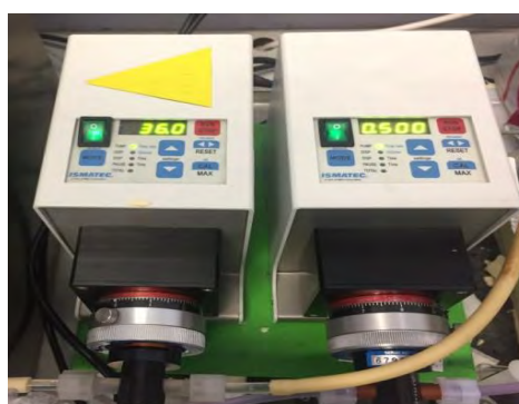
Figure 7.7: Peristaltic pumps used to feed chemical to maintain 500mg/l calcium carbonate concentration throughout experiment.
