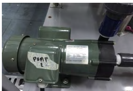
Figure 3.13: Araki EX-100RM magnetic driven seal-less chemical pump.
