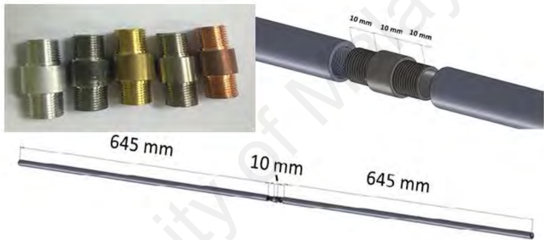
Figure 4.2: Coupons installation of different materials on heat exchanger surfaces.
