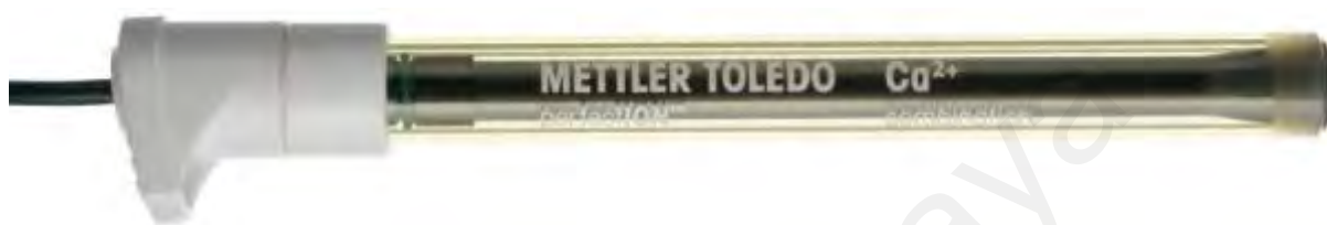
Figure 7.6: PerfectION combination calcium electrode used in our experimental set-up (Athavale et al., 2017).
