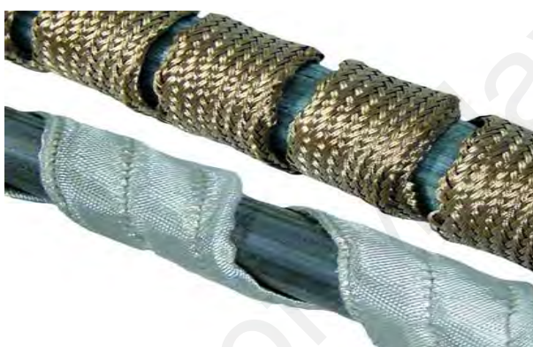
Figure 7.5: High temperature heating tapes wrapping around test section for constant heat flux (Edwards & Bindra, 2017).
