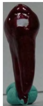
Figure 3.4: Varnished tooth with an unvarnished window area of 2 mm x 2 mm
