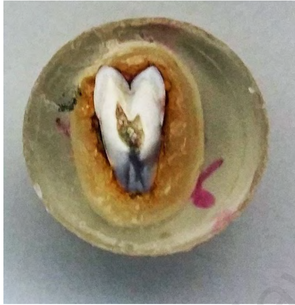
Figure 3.6: Picture showing the longitudinal section of a tooth mounted on epoxy resin
