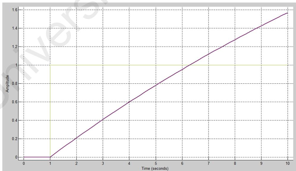
Figure 4.7: Open loop system response to step input in 10s (water level control with mathematical modelling data)
