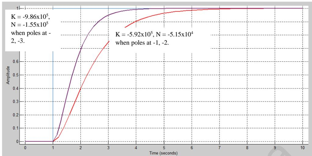
Figure 4.16: State feedback with tracking control/integral action (liquid level control with HYSYS modelling data)
