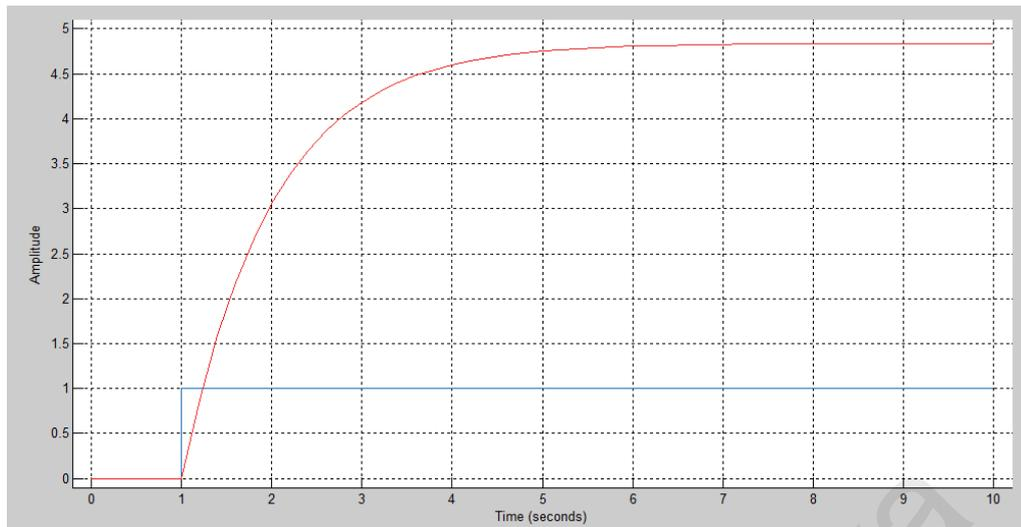
Figure 4.21: State feedback controller with feedforward gain (water level control with HYSYS modelling data)
