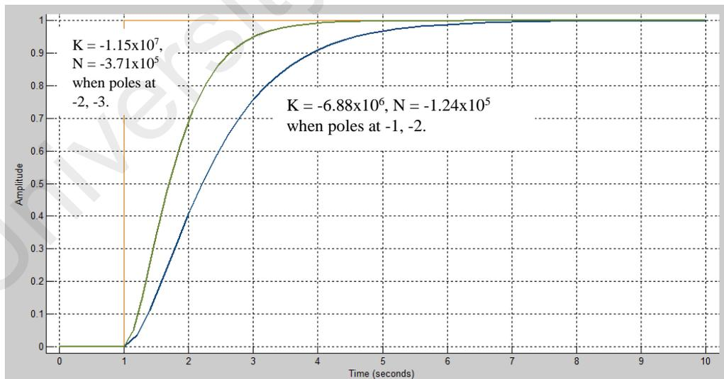
Figure 4.22: State feedback with tracking control/integral action (water level control with HYSYS modelling data)
