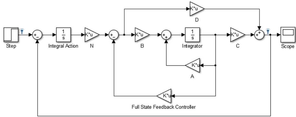
Figure 3.10: State feedback tracking controller
