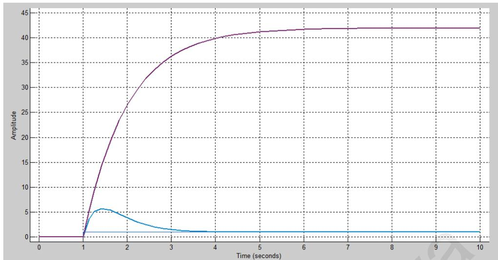
Figure 4.23: Disturbance rejection of system with and without integral action (water level control with HYSYS modelling data)
