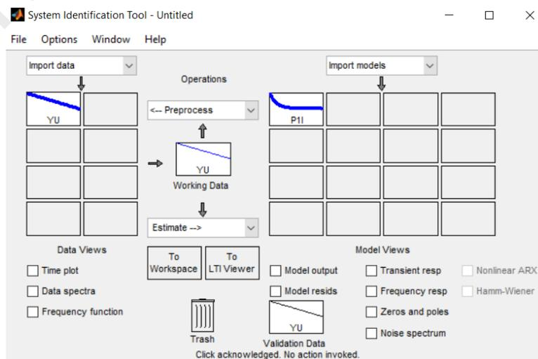
Figure 3.4: System Identification Tool to generate state space model for liquid level state variable
