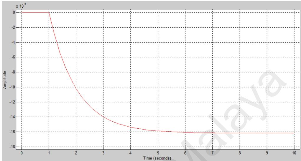
Figure 4.20: Full state feedback controller (water level control with HYSYS modelling data)
