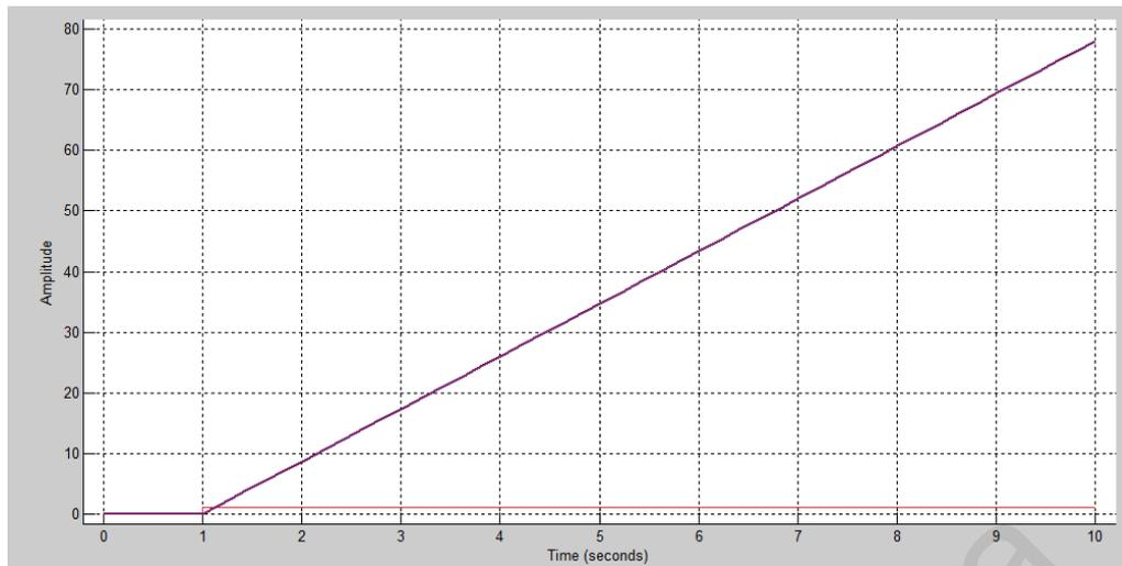
Figure 4.18: Disturbance rejection of system without integral action (liquid level control with HYSYS modelling data)
