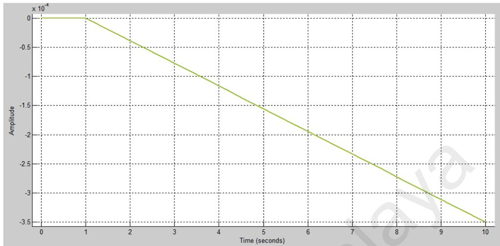
Figure 4.13: Open loop system response to step input (liquid level control with HYSYS modelling data)
