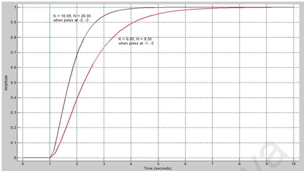
Figure 4.11: State feedback tracking control/integral action (water level control with mathematical modelling data)
