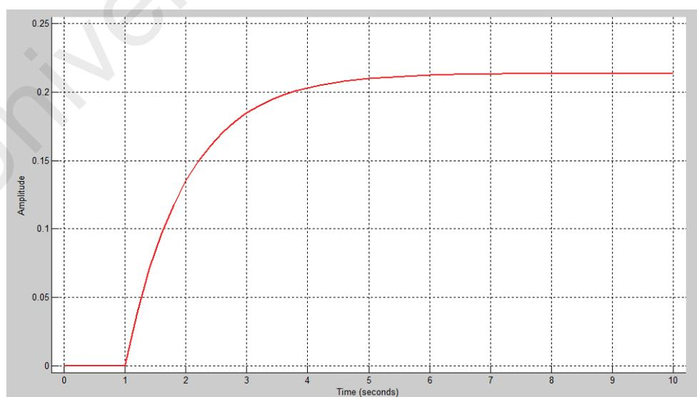
Figure 4.9: Full state feedback controller (water level control with mathematical modelling data)
