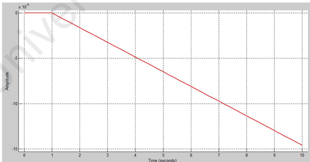
Figure 4.19: Open loop system response to step input (water level control with HYSYS modelling data)
