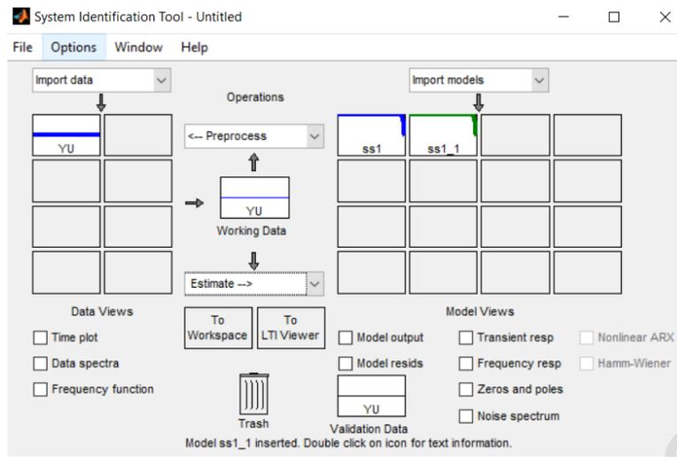
Figure 3.6: System Identification Tool to generate state space model for water level state variable
