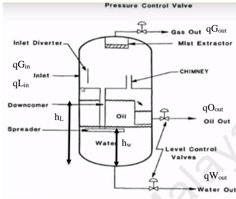
Figure 3.1: Schematic diagram of vertical three-phase separator
