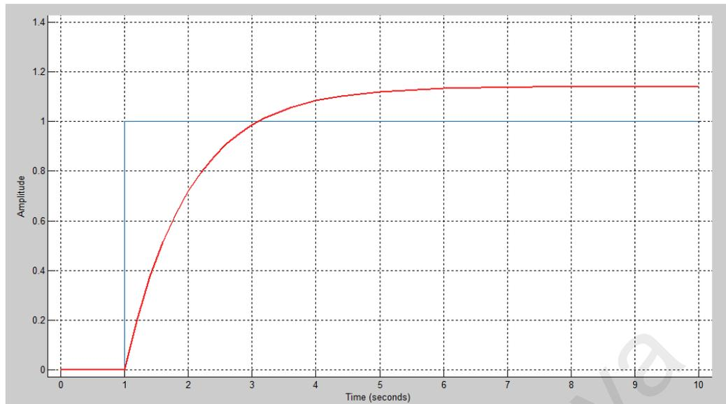
Figure 4.4: State feedback controller with feedforward gain (liquid level control with mathematical modelling data)
