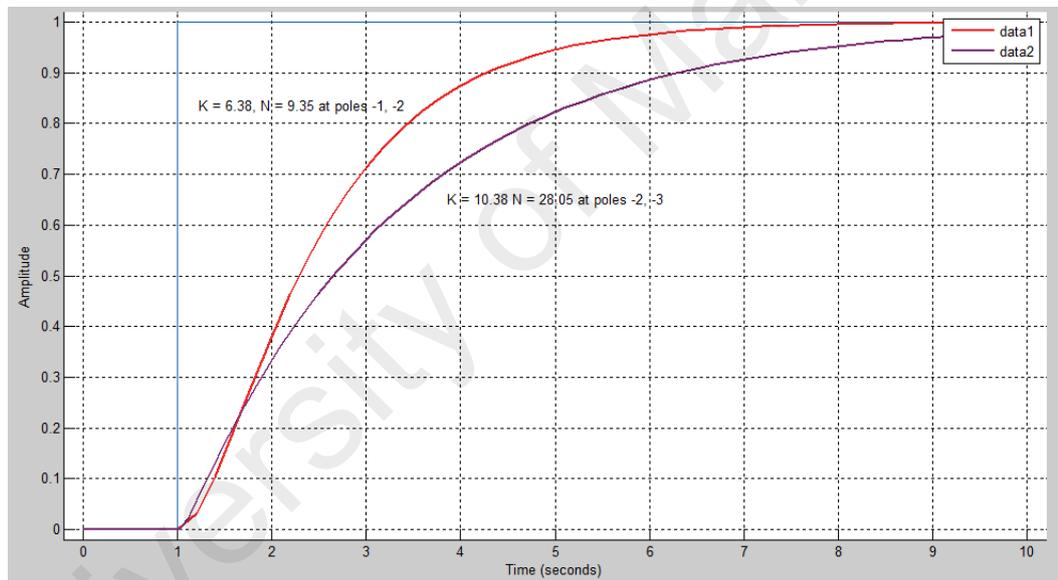
Figure 4.5: State feedback with tracking control/integral action (liquid level control with mathematical modelling data)
