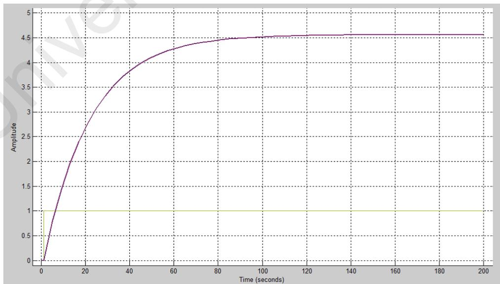
Figure 4.2: Open loop system response to set input in 200s (liquid level control with mathematical modelling data)
