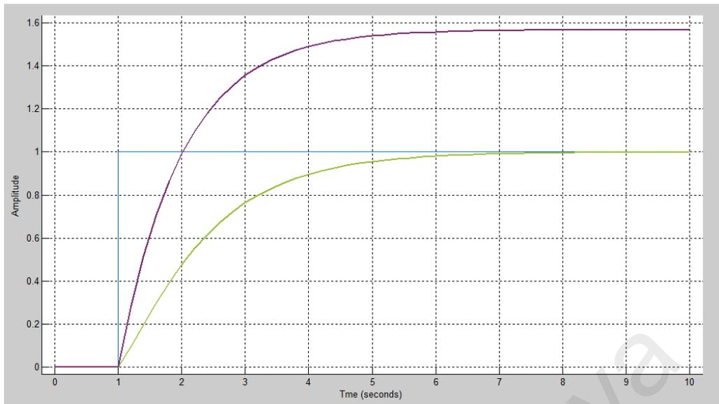
Figure 4.6: Disturbance rejection (liquid level control with mathematical modelling data)
