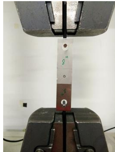
Figure 3.7: Schematic illustration of tensile shear test specimen
