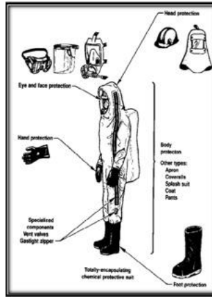
Figure 4.11: PPE recommended in the SOP for sampling activity
