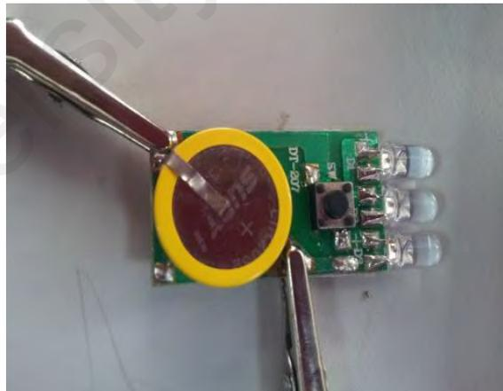
**Figure 4.12: The Storage Battery Circuit with Three LEDs**
