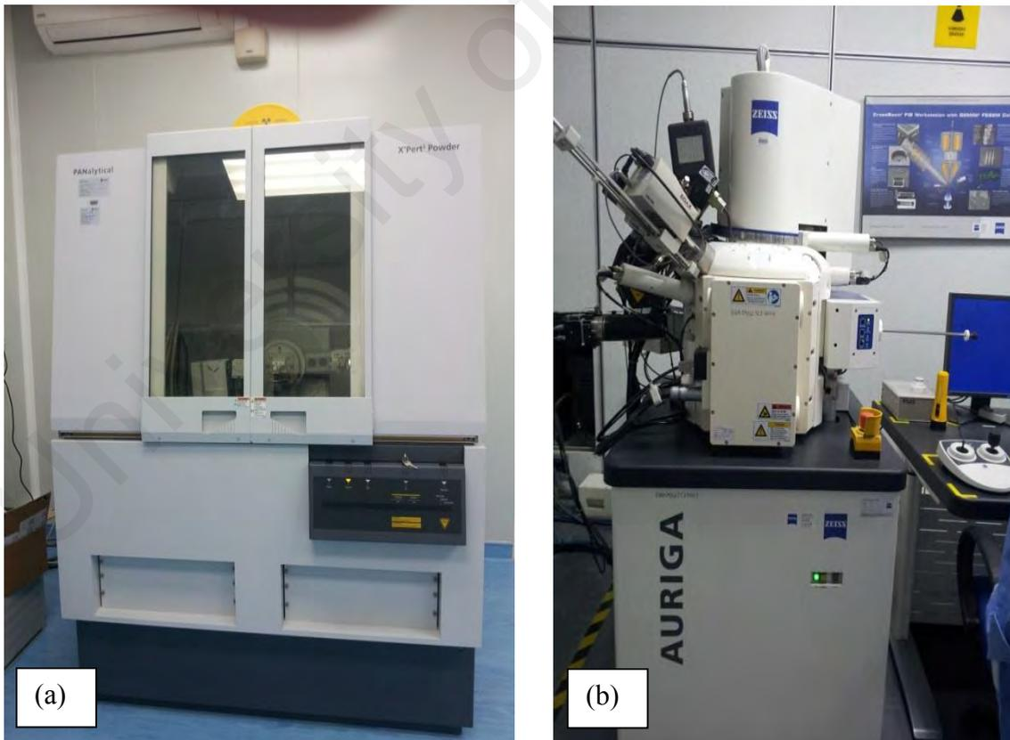
**Figure 3.4: (a) X-ray Diffraction System (PANalytical X'Pert3 X-ray Diffractometer), (b) Field Emission Scanning Electron Microscope (ZEISS Sdn. Bhd)**
