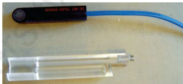
Figure 7.3: INTRABEAM water phantom provided for in-house QA procedure (picture taken from INTRABEAM® water phantom manual)
