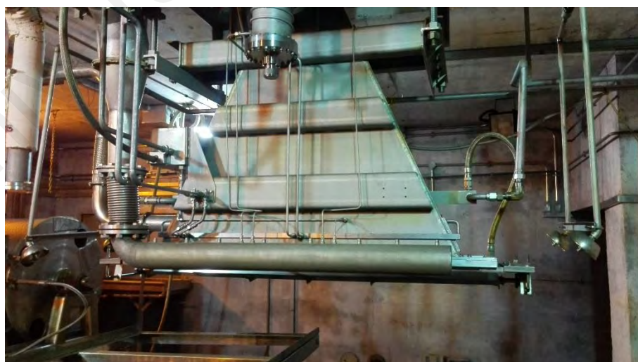
Figure 8.1: Output window of ALURTRON electron accelerator for industrial radiation processing
