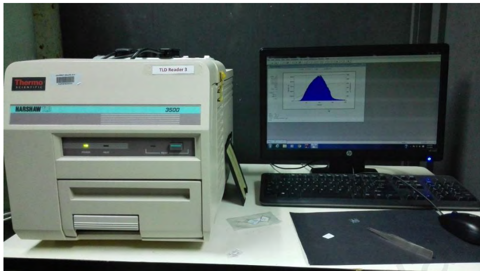
Figure 3.4: Harshaw 3500 TLD reader connected to WinREMS software
