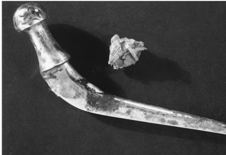
Figure 2.3: Corrosion failure of SS Hip joint stem implant (Q. Chen & Thouas, 2015)
