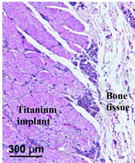
Figure 2.11: infusion at the interface between bone and Ti implant (Q. Chen & Thouas, 2015)
