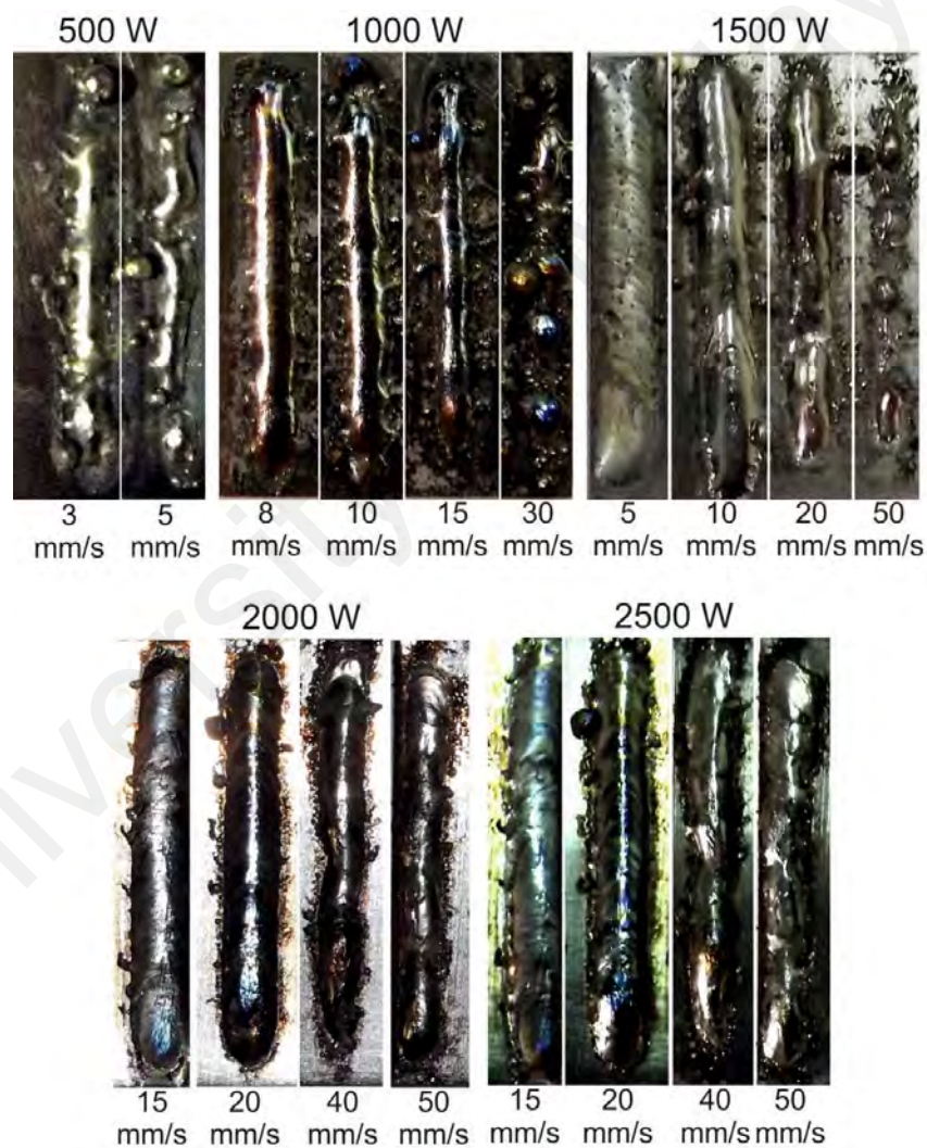
Figure 4.1: Morphology of single cladded tracks
