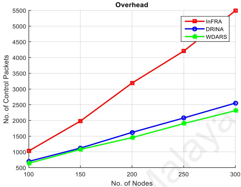
**Figure 4.11: Overhead Comparison for Different Node Quantities**
