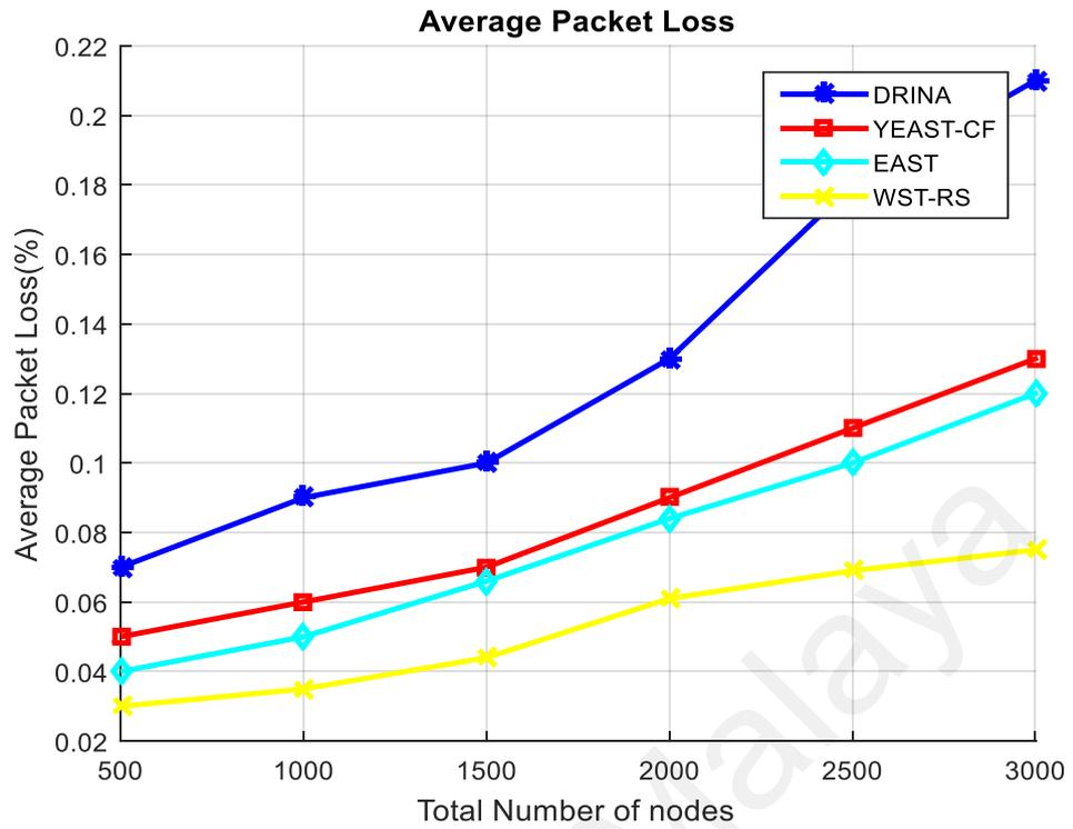
**Figure 5.10: Comparison of the Average Packet Loss Rates in Scenario I**
