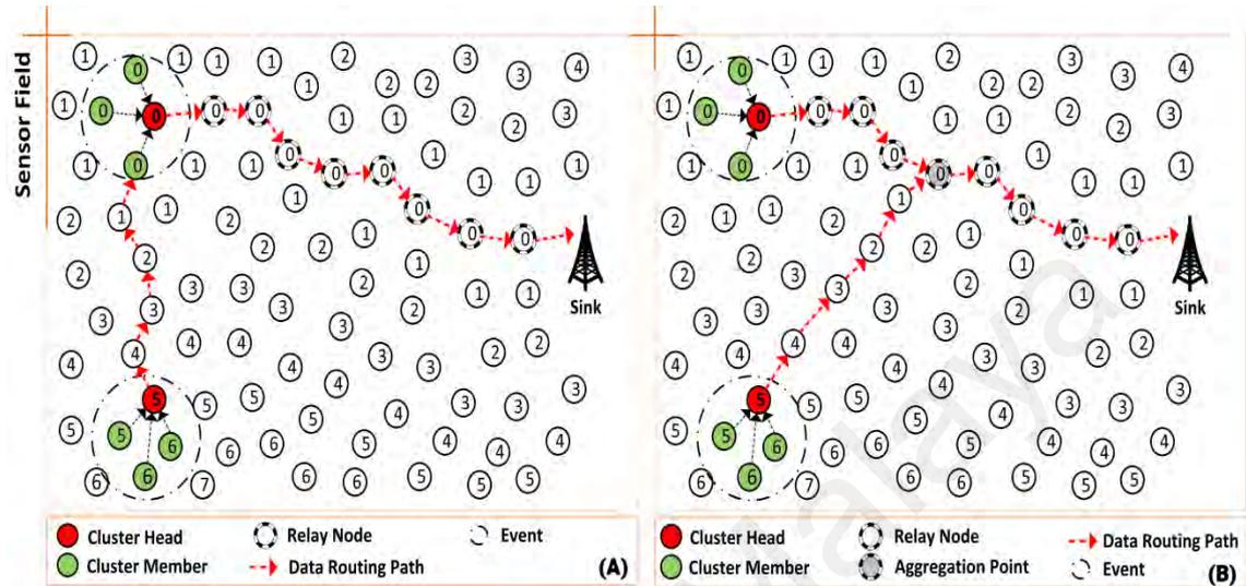
**Figure 4.4: A Comparison of the New Path Formation Processes of (A) DRINA and (B) WDARS**
