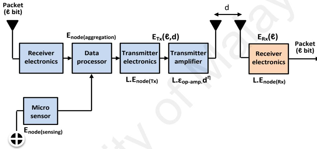
Figure 3.5: Energy Consumption Model
