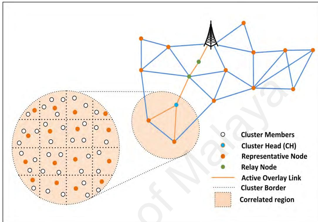
**Figure 5.3: Network Model Diagram of WST-RS for Routing to the Sink Node**
