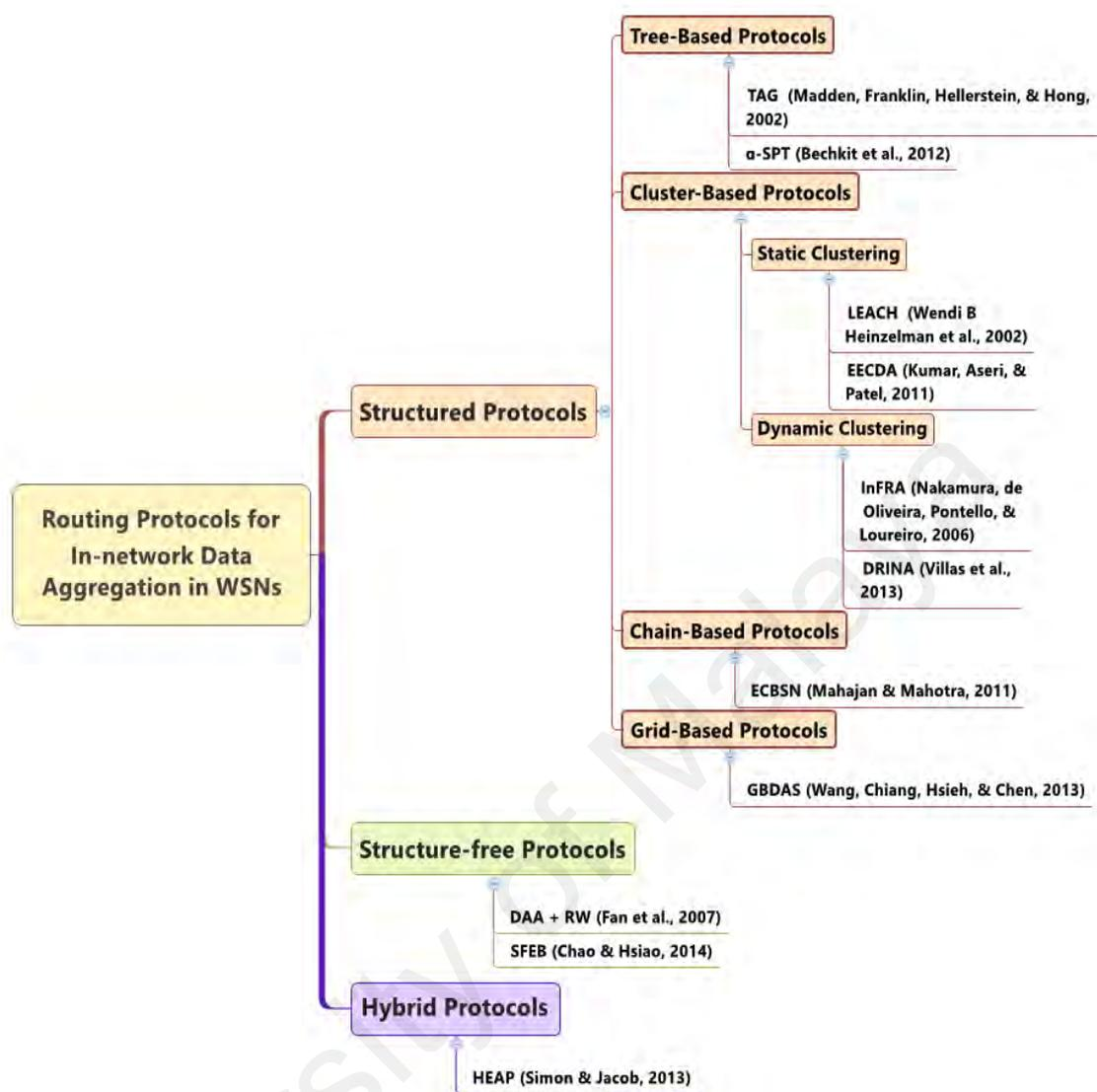
**Figure 2.3: Classification of Routing Protocols for In-Network Data Aggregation in WSNs**
