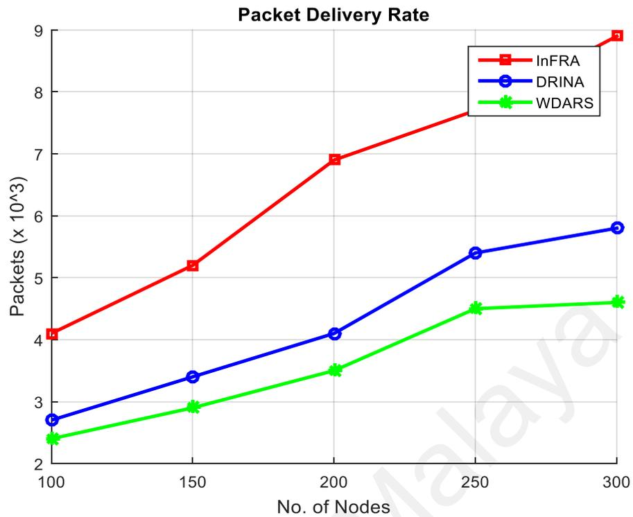
**Figure 4.9: Comparison of the Packet Delivery Rates for Different Node Quantities**
