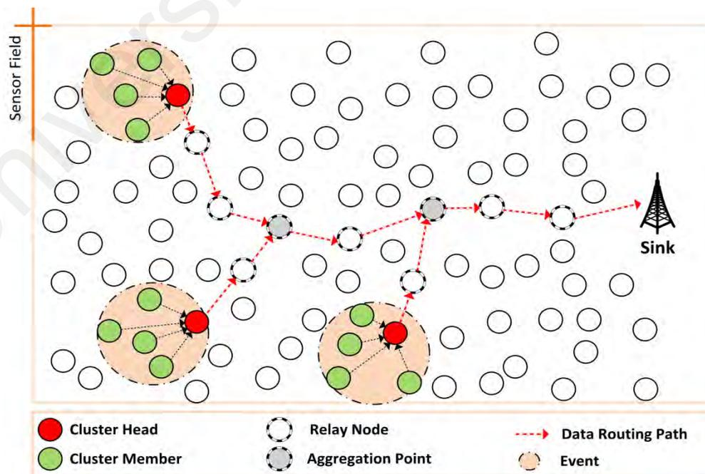
**Figure 4.1: Diagram of the Network Model of WDARS for Routing to the Sink Node**
