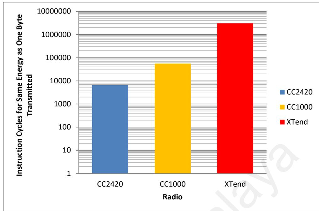
**Figure 1.2: CPU Compute Cycles Versus Transmission Energy of One Byte Over Three Radios**
