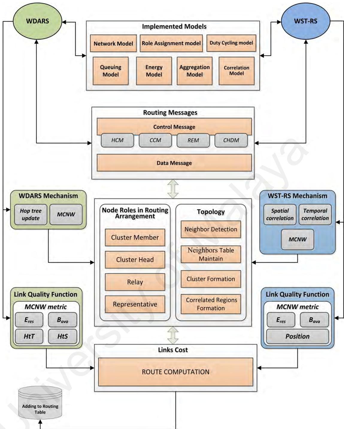
**Figure 3.4: Architecture of Implemented Proposed Schemes**
