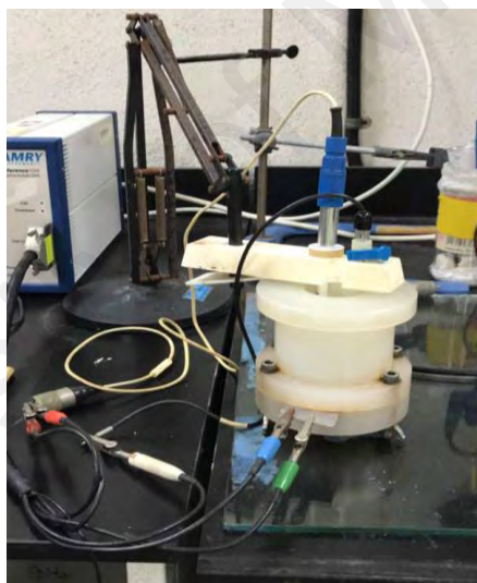
Figure 3.4: Three electrode system set up for electrochemical analysis
