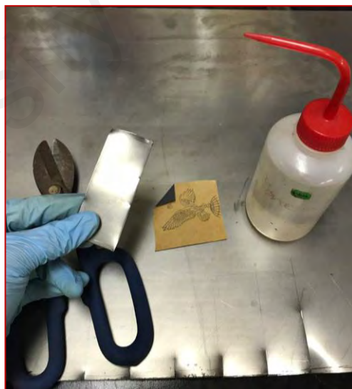
Figure 3.3: Preparation of mild steel specimens.
