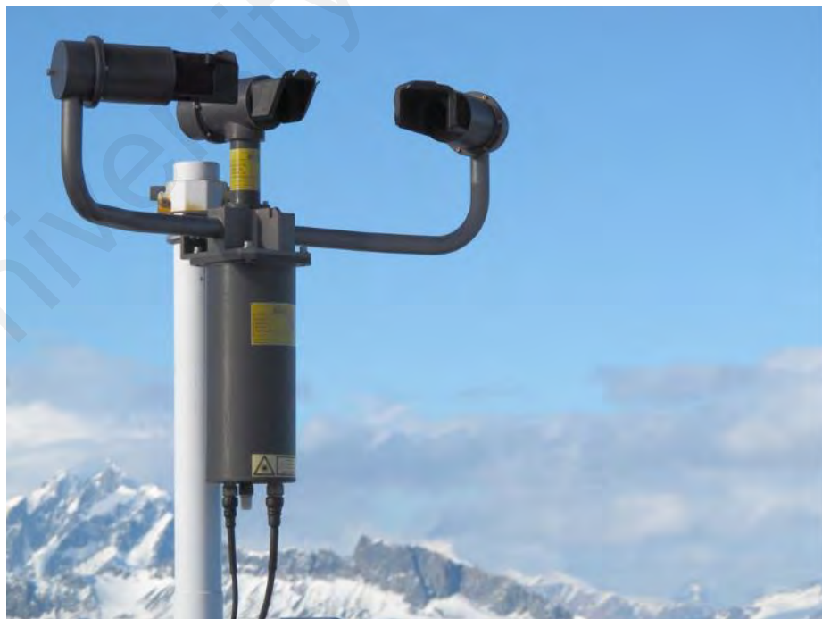
Figure 3.3 The VPF-730 system installed at Rothera.
