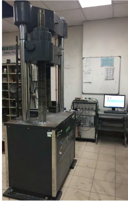
Figure 5.6: The IPC UTM-1000 used for the tensile test
