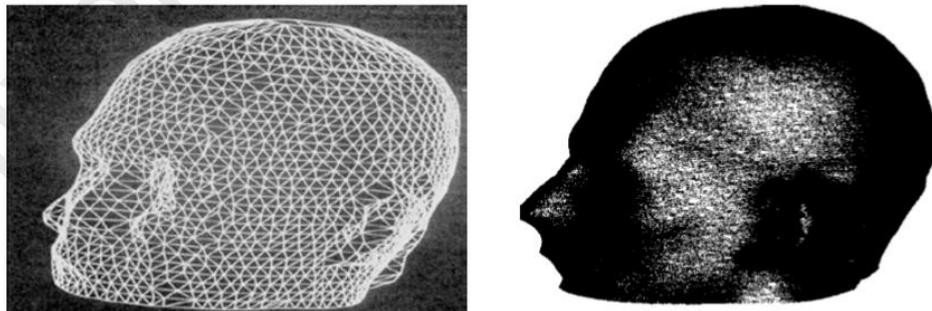
**Figure 17 (left) Optimal tiled surface defined over the contours; (right) 3D reconstruction of face**
