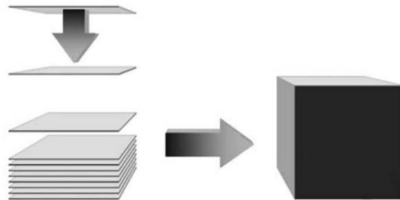
**Figure 1** The representation of the images in a virtual 3D space in their respective position produces a cube of data. Images are bidimensional and spaced. The gaps of missing data can be filled through interpolation of the values of the images. In this way, a solid cube of data is obtained. This 3D cube of data is made of elementary units, which are referred as to volume elements (voxels)
