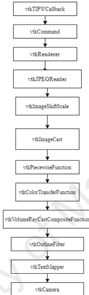
**Figure 23 Pipeline for volume rendering with measurement feature**
