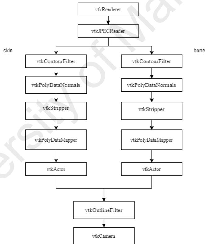
**Figure 20 Pipeline for surface rendering method**
