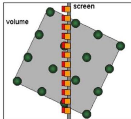
**Figure 8 Multiplanar reformation. In multiplanar reformation, the points of the plane crossing the volume are obtained by interpolation from the known points of the volume. Red squares: interpolated points; yellow square: pixel; green circles: points of the volume (voxels)**
