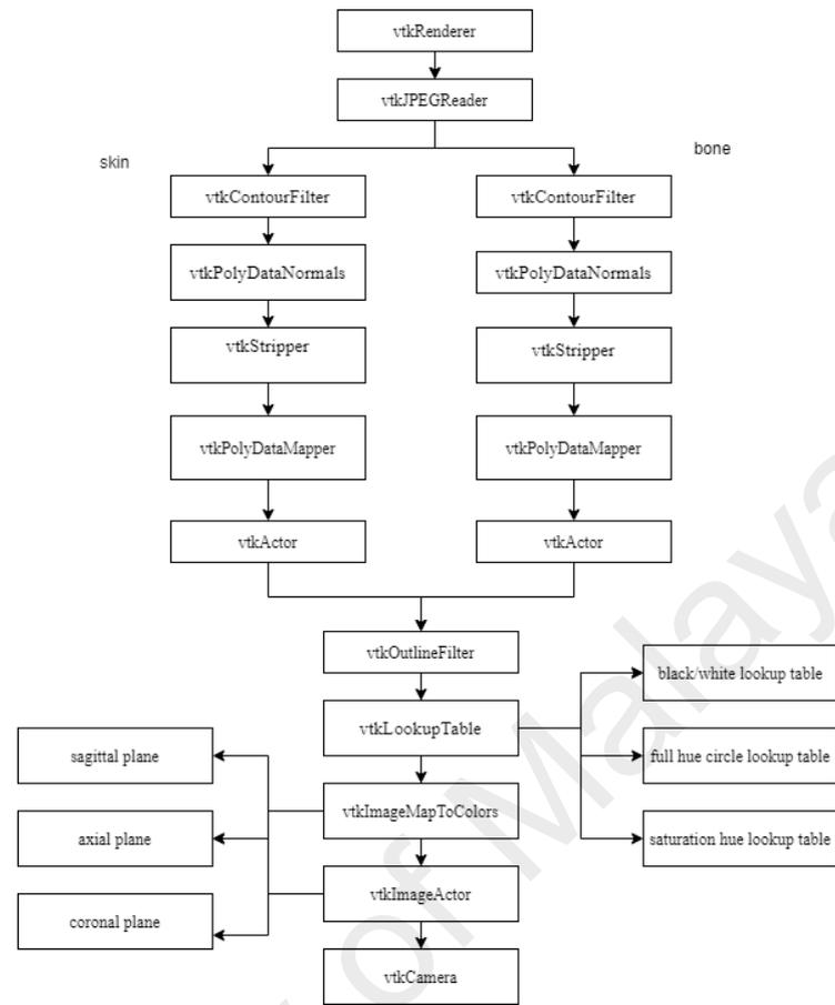
**Figure 21 Surface rendering and multi multiplanar rendering method**
