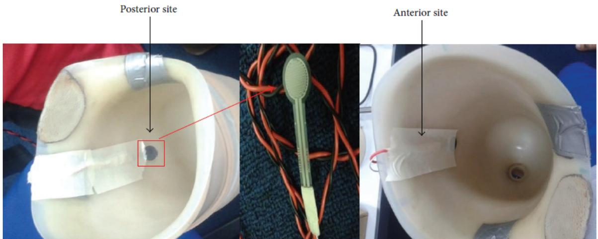
**Figure 2.8: Locations of FSRs attached to the socket's wall(El-Sayed et al., 2015)**
