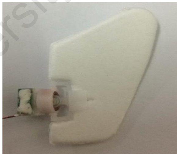
Figure 3.14: Magnetic actuator for flight control
