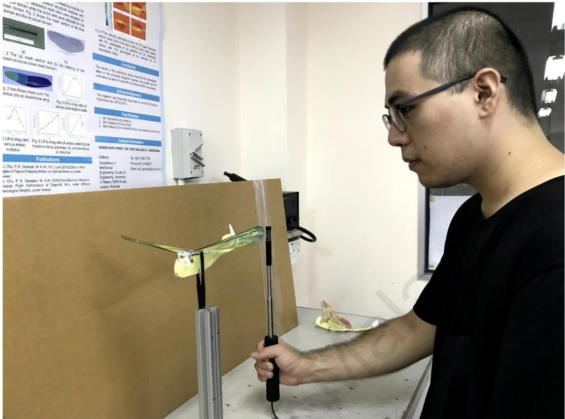
**Figure 3.14 Measurement of velocity generated by wings**
