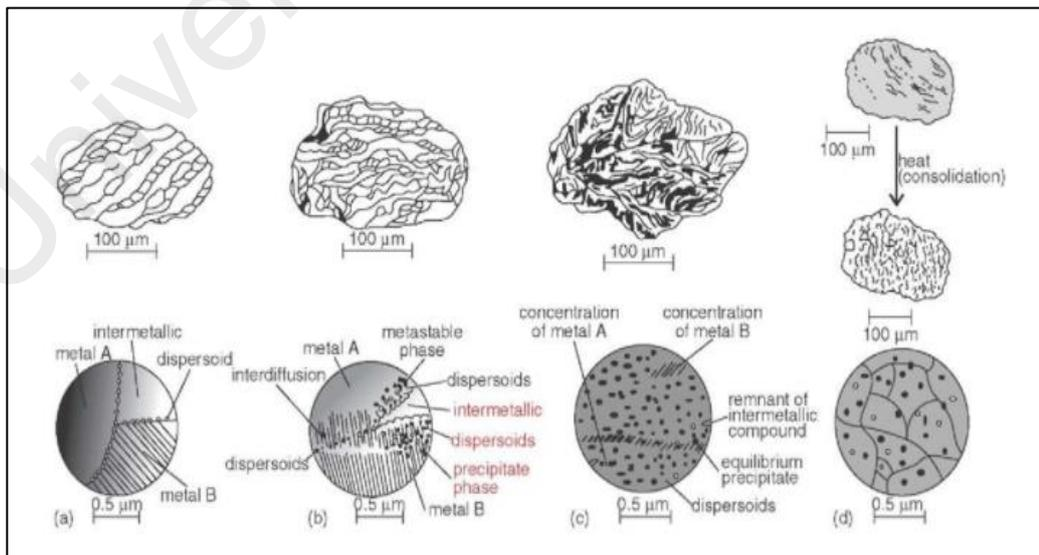
Figure 2.3 : Illustration of Mechanical Alloying
