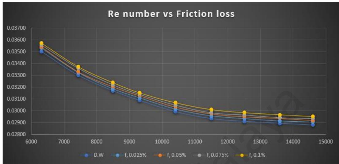
**Figure 4.4 : Re number against Friction Loss**
