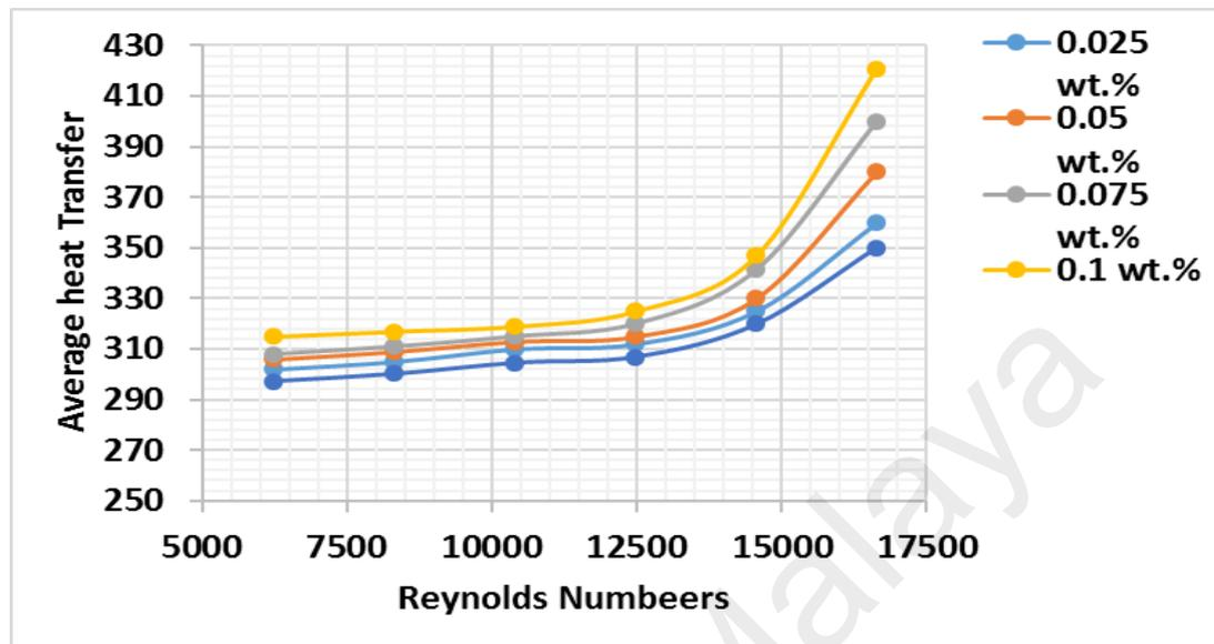
**Figure 2.12: Re number against Heat Transfer Coefficient**
