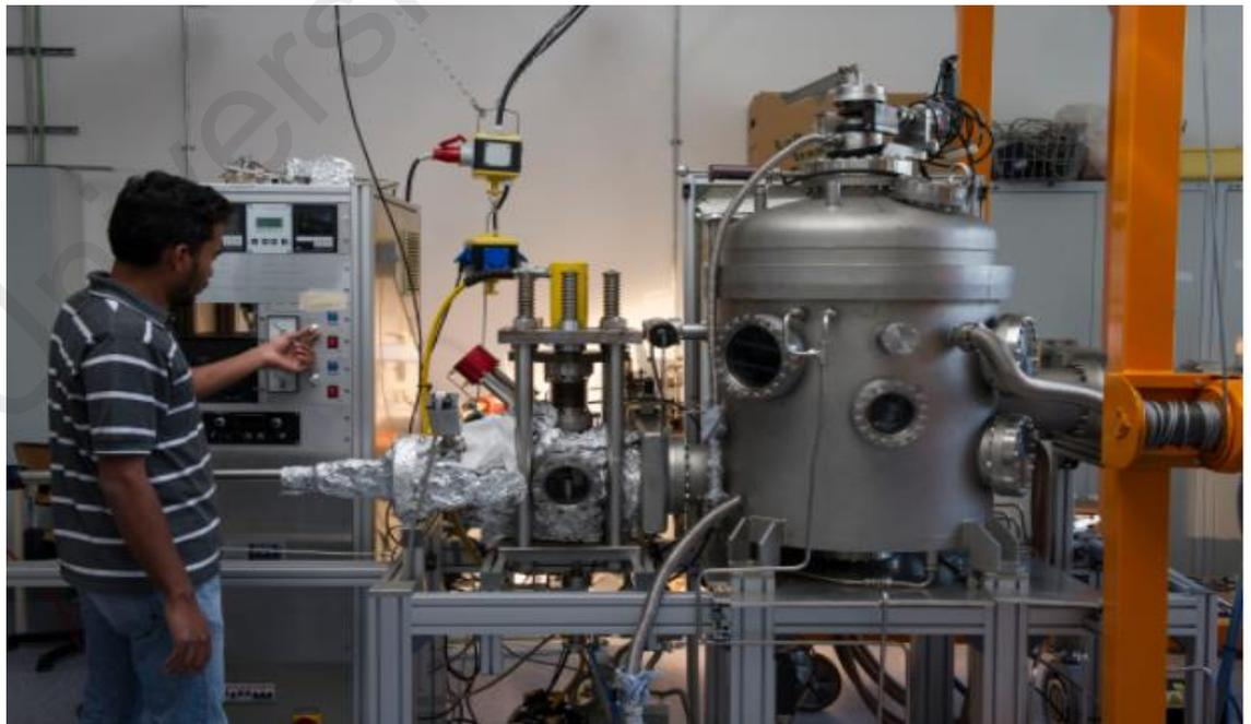
**Figure 2.1: Image of Inert Gas Condensation**
