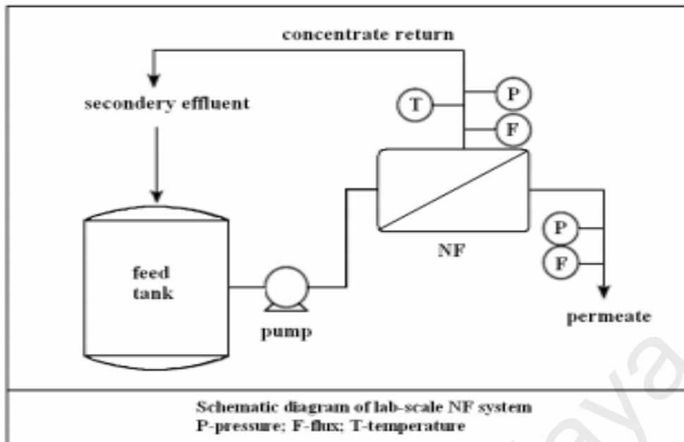
**Figure 2.10 : Schematic diagram of lab-scale NF system**
