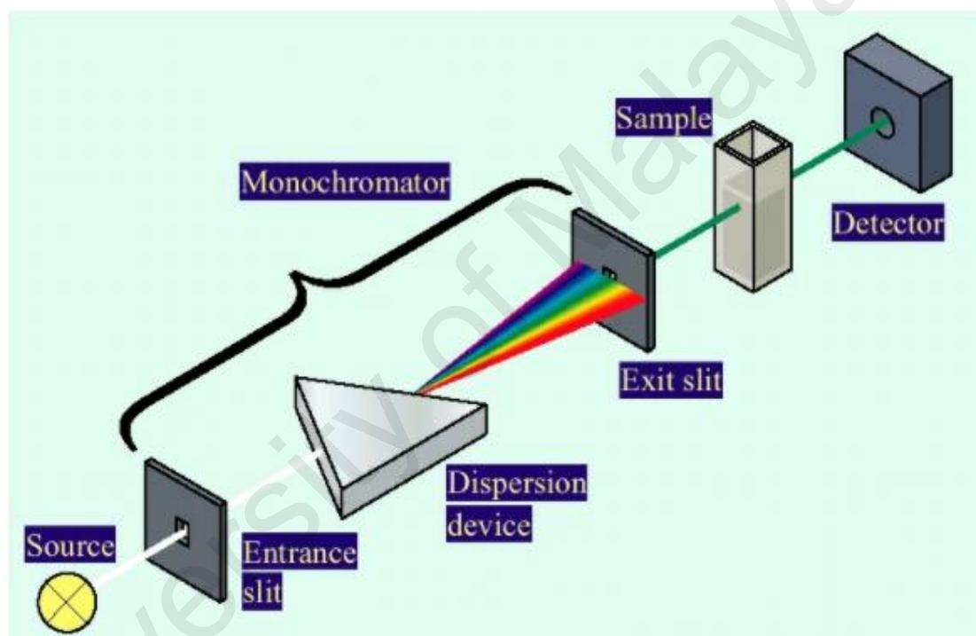
**Figure 2.6 : Function of UV-vis spectrophotometer**
