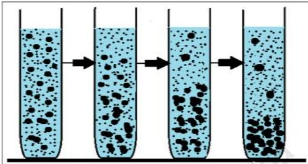
**Figure 2.4 : Sedimentation Process**
