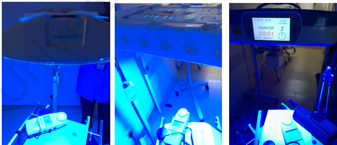
Figure 3.4: Measurement of irradiance for each type of phototherapy light devices
