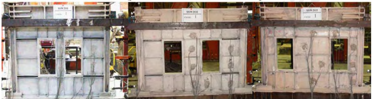
Figure 2-30 Stiffened SPSW with two rectangular perforation tested by (Sabouri-Ghomi and Mamazizi, 2015)
