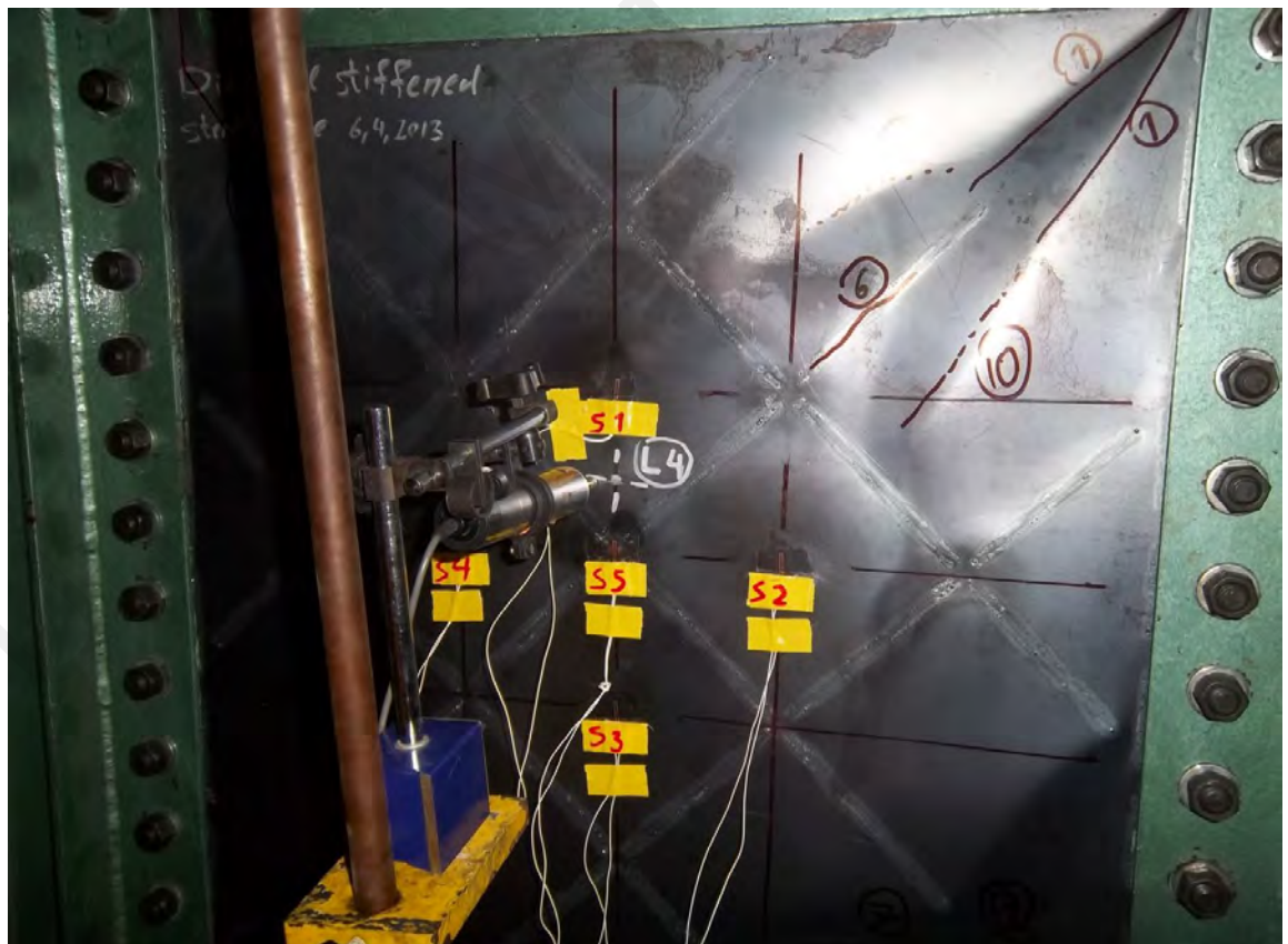
Figure 3-47 Nodal buckling line of DS-SPSW
