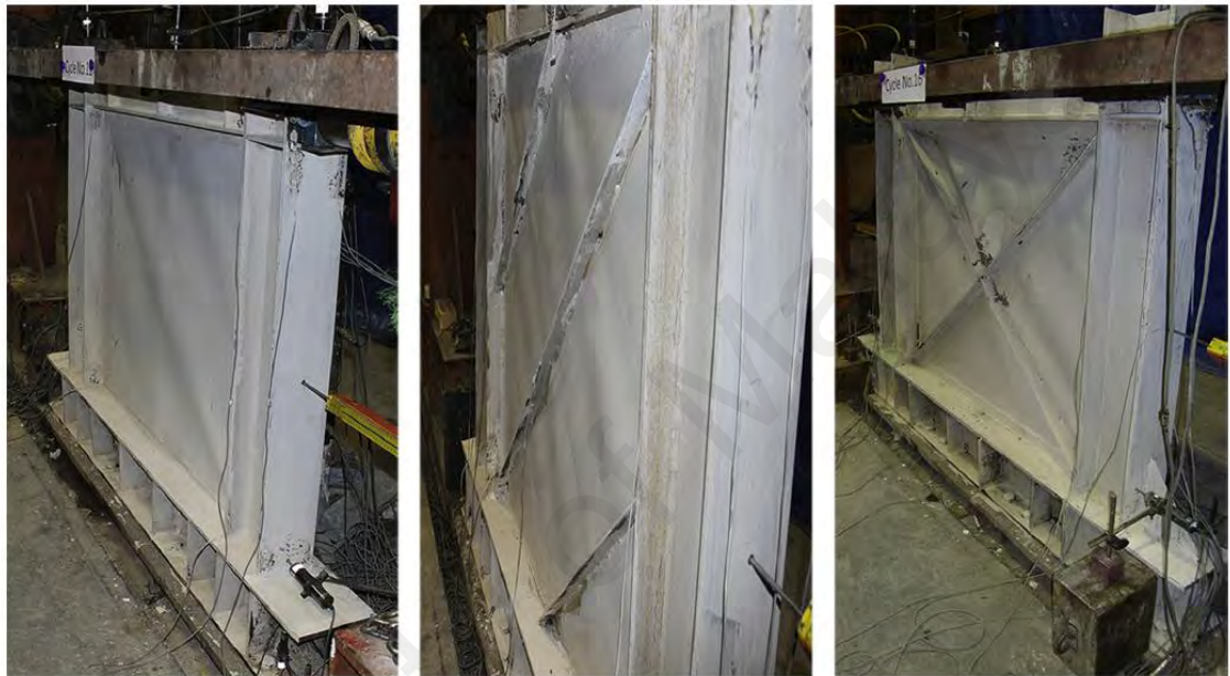
Figure 2-35 Unstiffened and diagonally stiffened specimens of Sigariyazd, et al. (2016)
