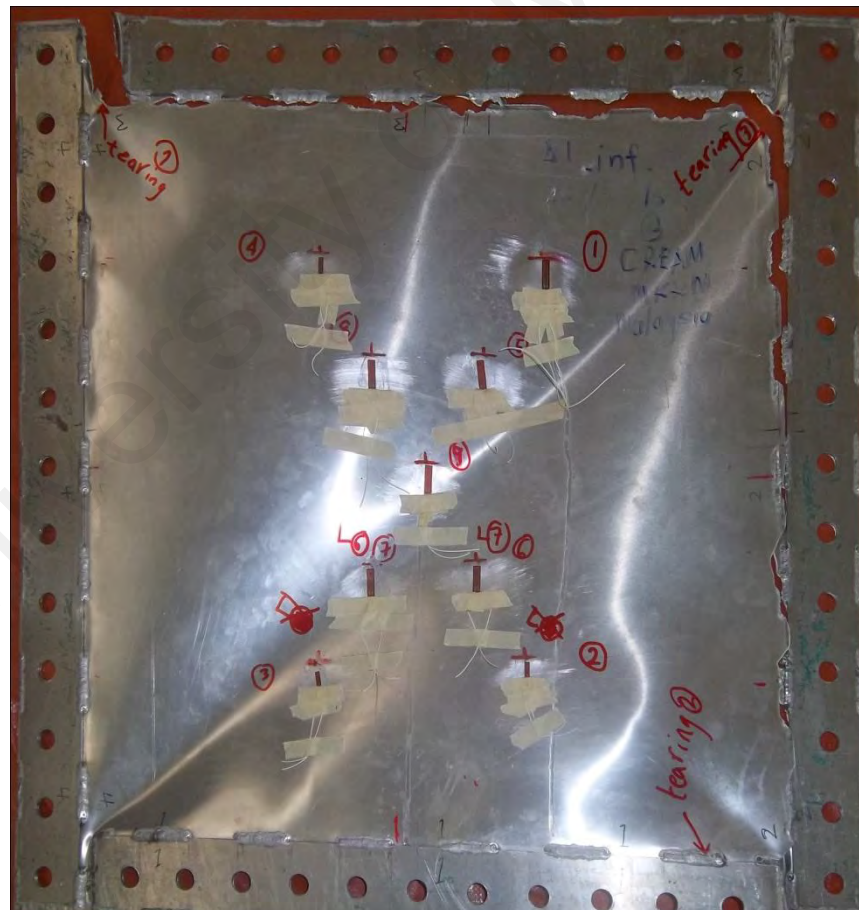
Figure 3-25 AL-SPSW after test
