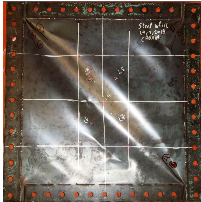
Figure 3-26 US-SPSW after test
