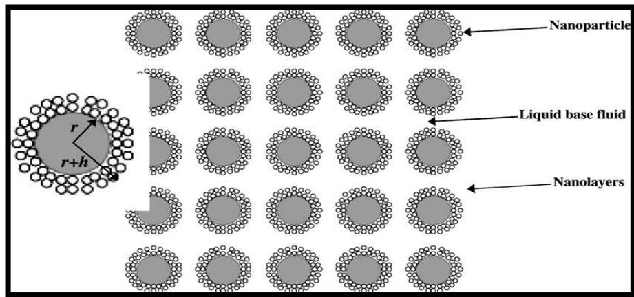
**Figure 2.9 : Schematic cross section of nanofluids structure
