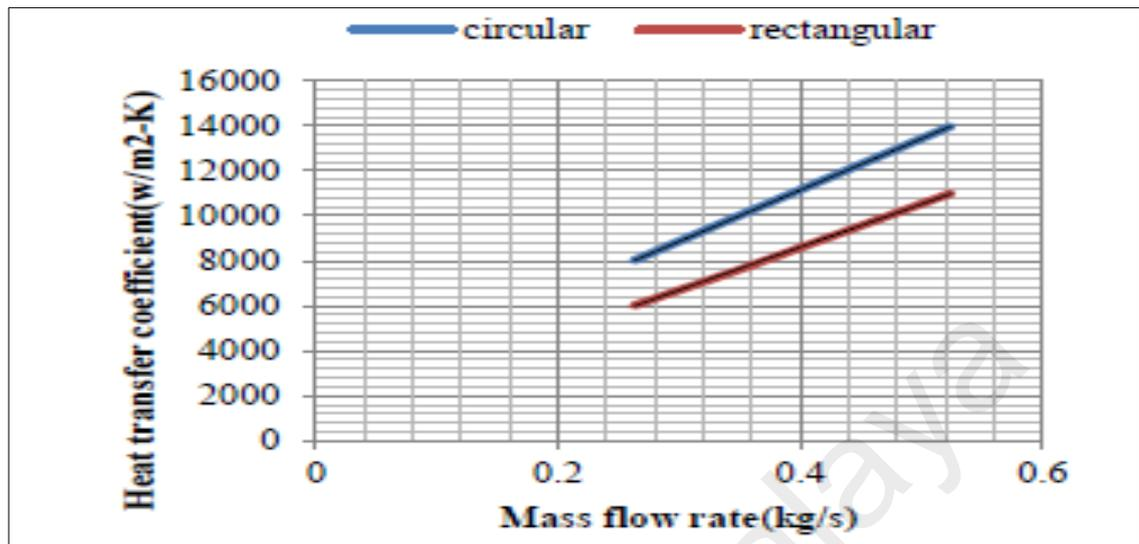
Figure 2.3 : Heat Transfer Coefficient vs Flow Rate
