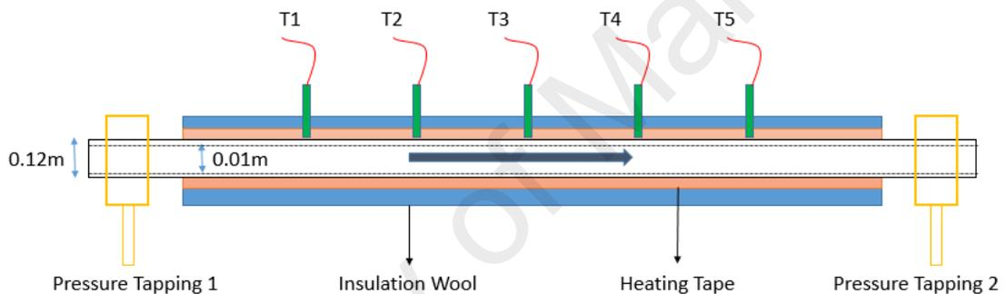
**Figure 3.4 : Sectional view of experimental test section**
