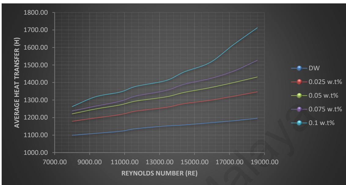
**Figure 4.1 : Average heat transfer coefficient at various Reynolds number**
