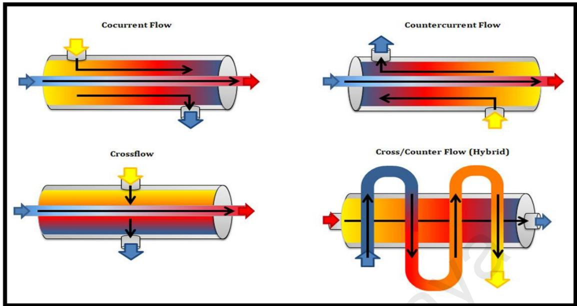
**Figure 2.1 : Heat exchanger flow configurations**
