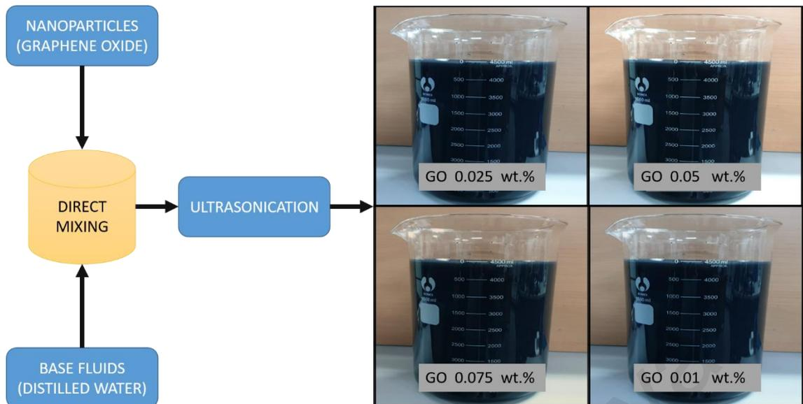
**Figure 3.2 : Two-step preparation process of nanofluids (Mukherjee & Paria, 2013)**
