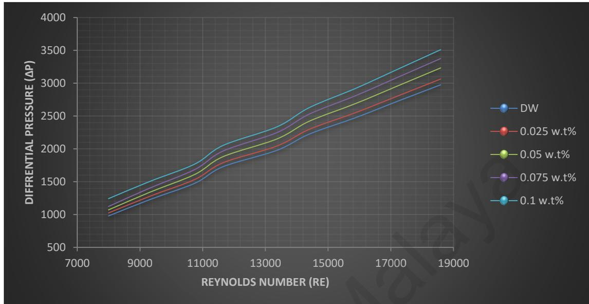
**Figure 4.3 : Pressure drop at various Reynolds number**
