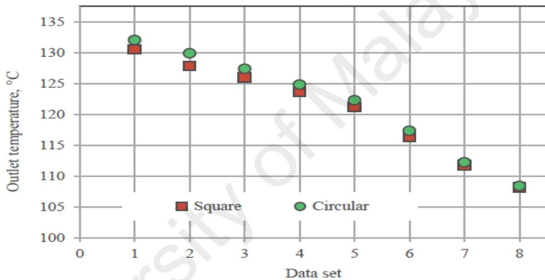
**Figure 2.4 : Effects of cross-section on heat transfer enhancement**
