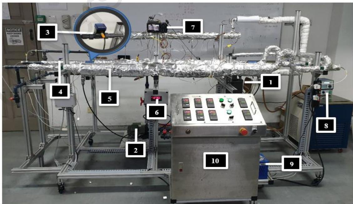
**Figure 3.3 : Rig used for convective heat transfer measurement**
