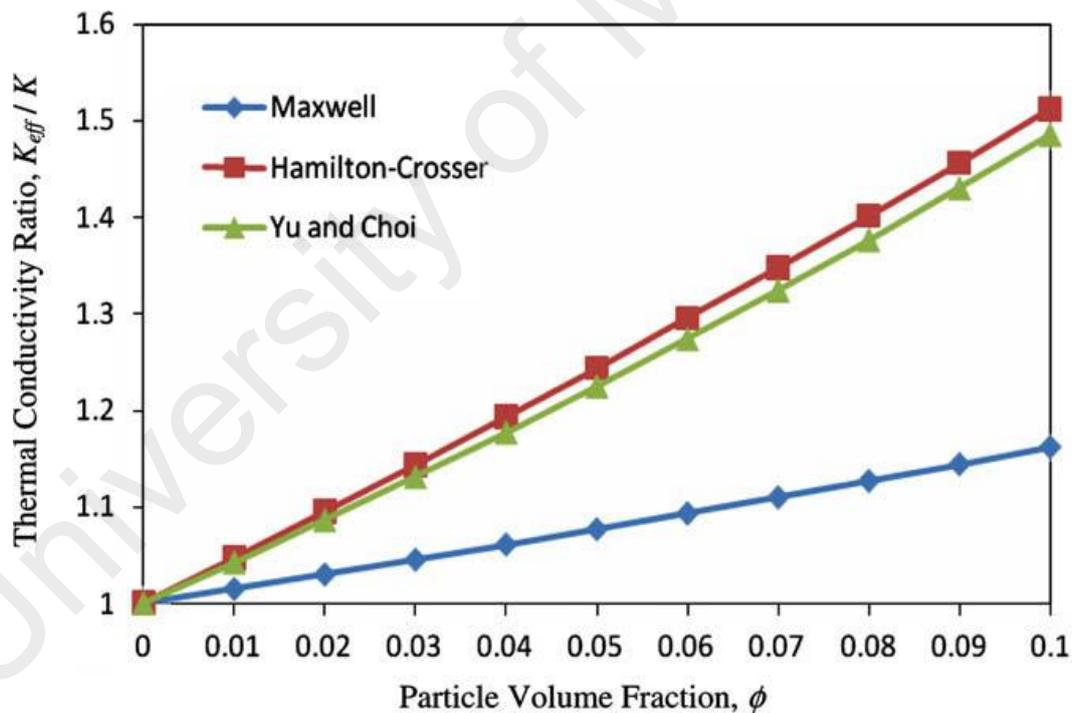
**Figure 2.10 : Variation of thermal conductivity ratio against particle volume fraction for  $\text{Al}_2\text{O}_3$ /water nanofluids**
