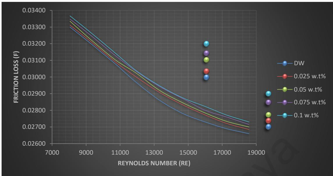
**Figure 4.4 : Friction loss at various Reynolds number**
