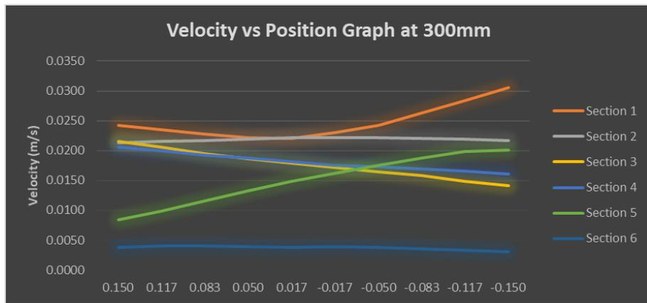
**Figure 4.13 Velocity vs Position Graph at 300mm of 6 sections of pipe**
