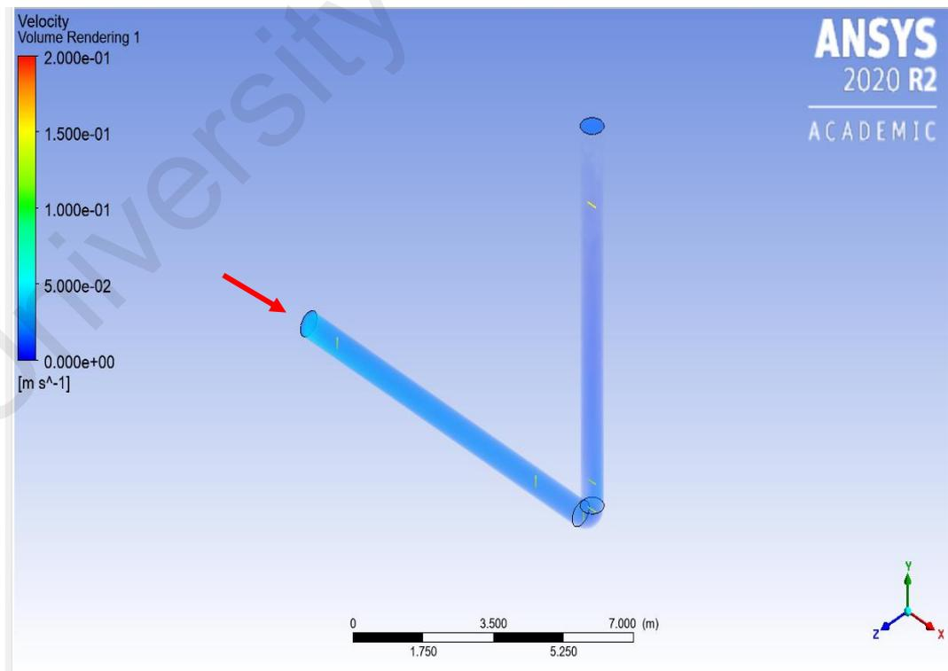
**Figure 4.3: Velocity contour of 300 mm diameter pipe**
