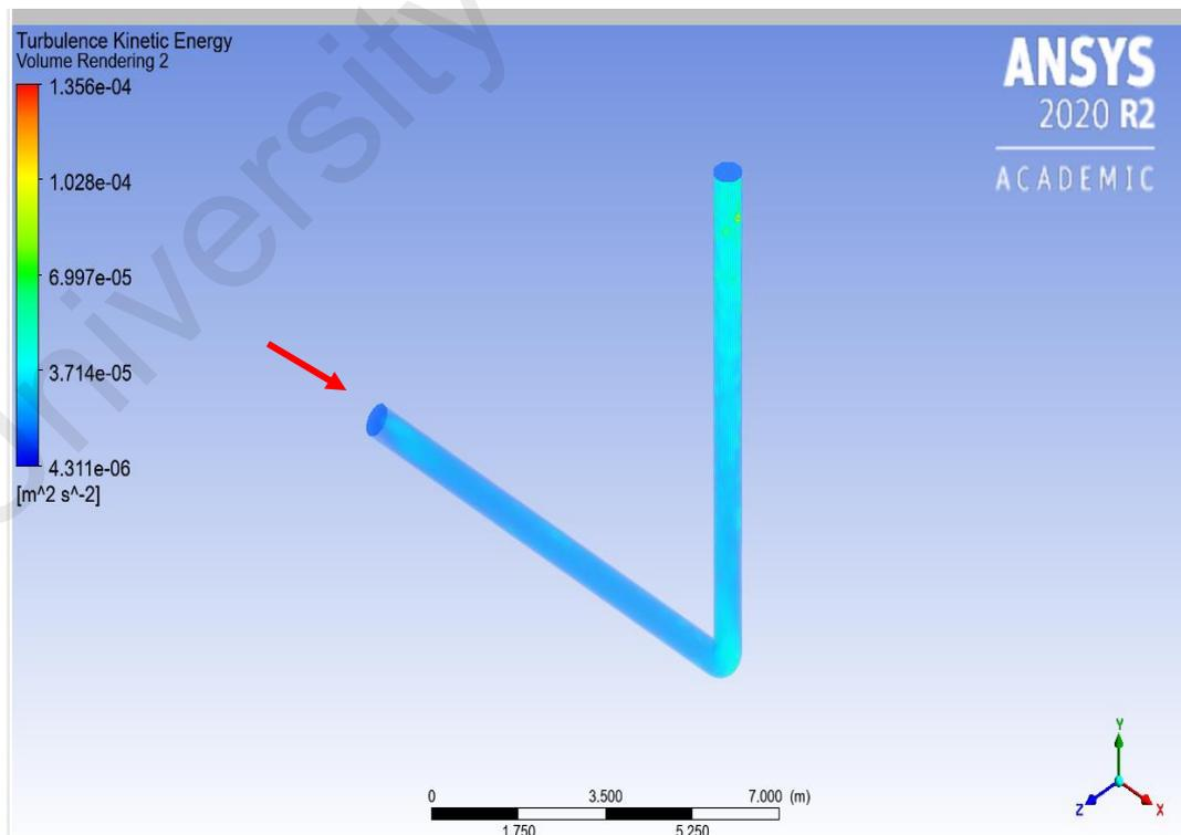
**Figure 4.8: Turbulence kinetic energy contour of 300 mm diameter pipe**
