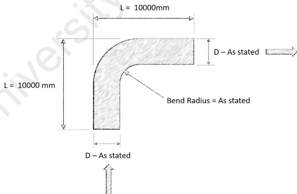
**Figure 3.1: Design of pipe constructed with 90 deg elbow**
