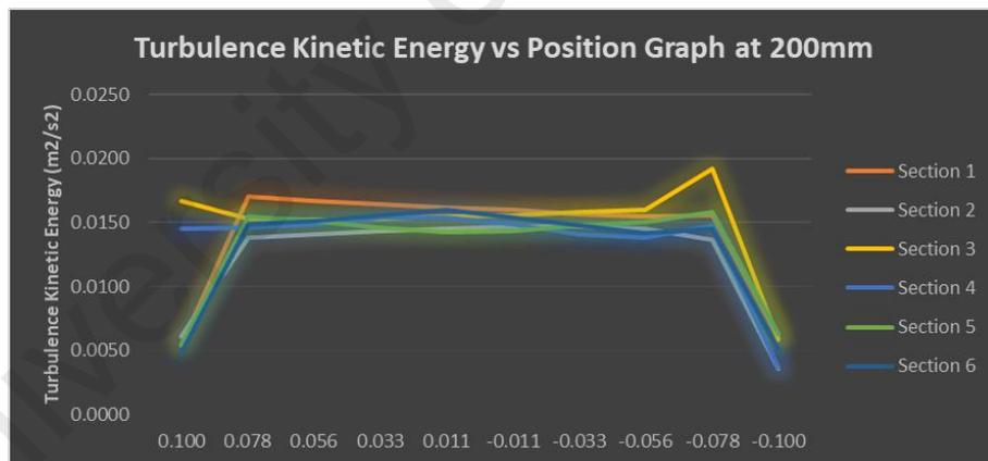
**Figure 4.16 Turbulence Kinetic Energy vs Position Graph at 200mm of 6 sections of pipe**
