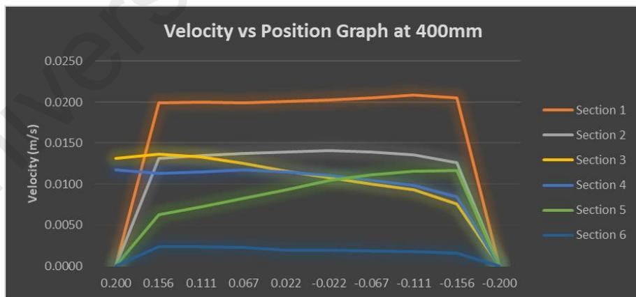
**Figure 4.15 Velocity vs Position Graph at 400mm of 6 sections of pipe**
