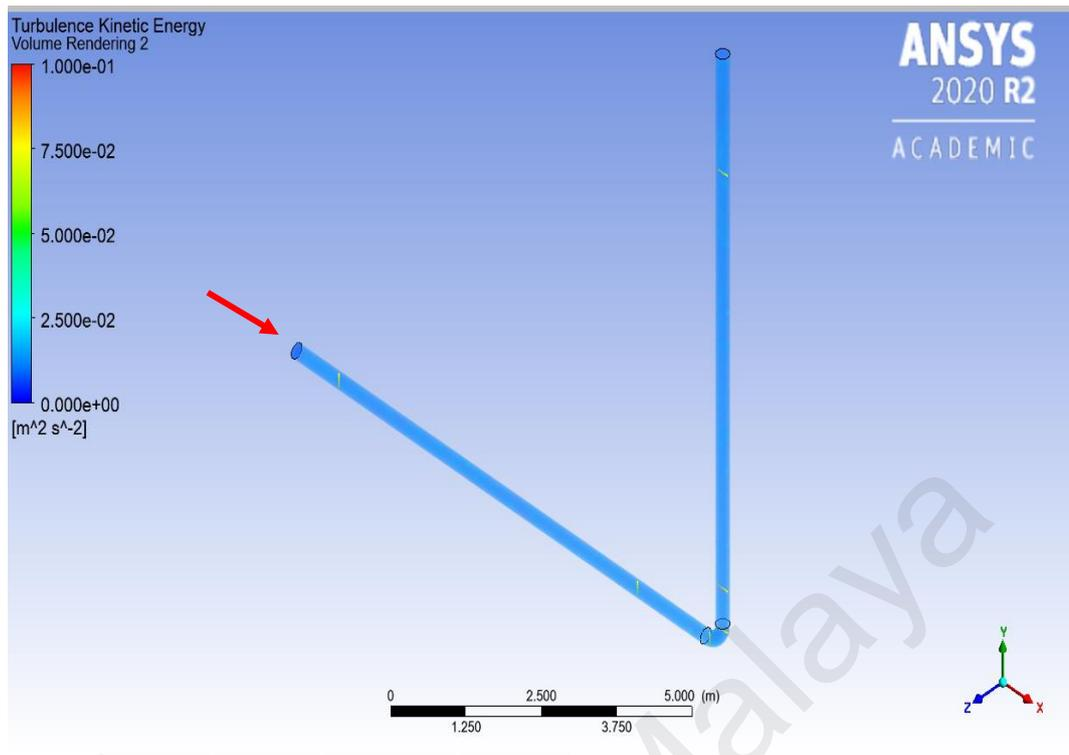
**Figure 4.7: Turbulence kinetic energy contour of 250 mm diameter pipe**
