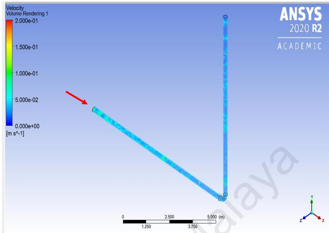
**Figure 4.2: Velocity contour of 250 mm diameter pipe**
