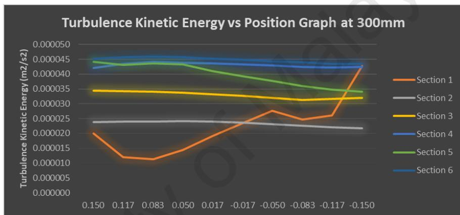
**Figure 4.18 Turbulence Kinetic Energy vs Position Graph at 300mm of 6 sections of pipe**
