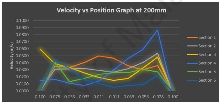
Figure 4.11 Velocity vs Position Graph at 200mm of 6 sections of pipe
