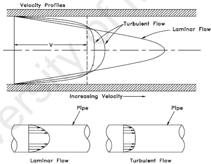
**Figure 2.2: Image of velocity profile related to flow**
