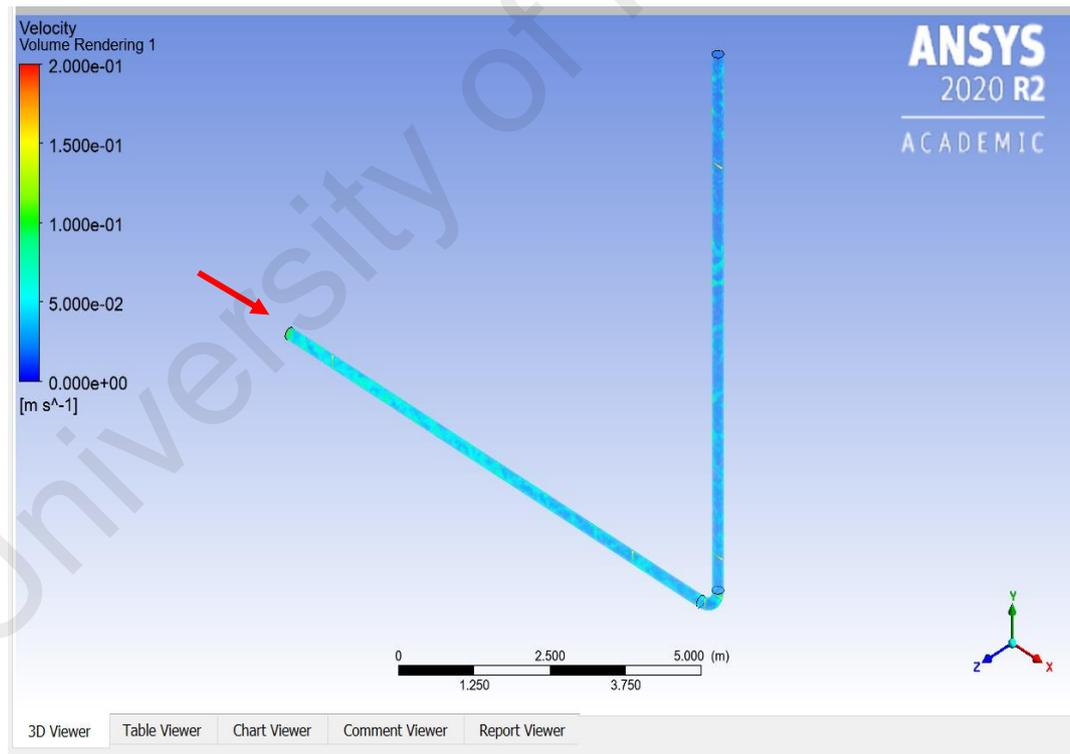
**Figure 4.1: Velocity contour of 200 mm diameter pipe**
