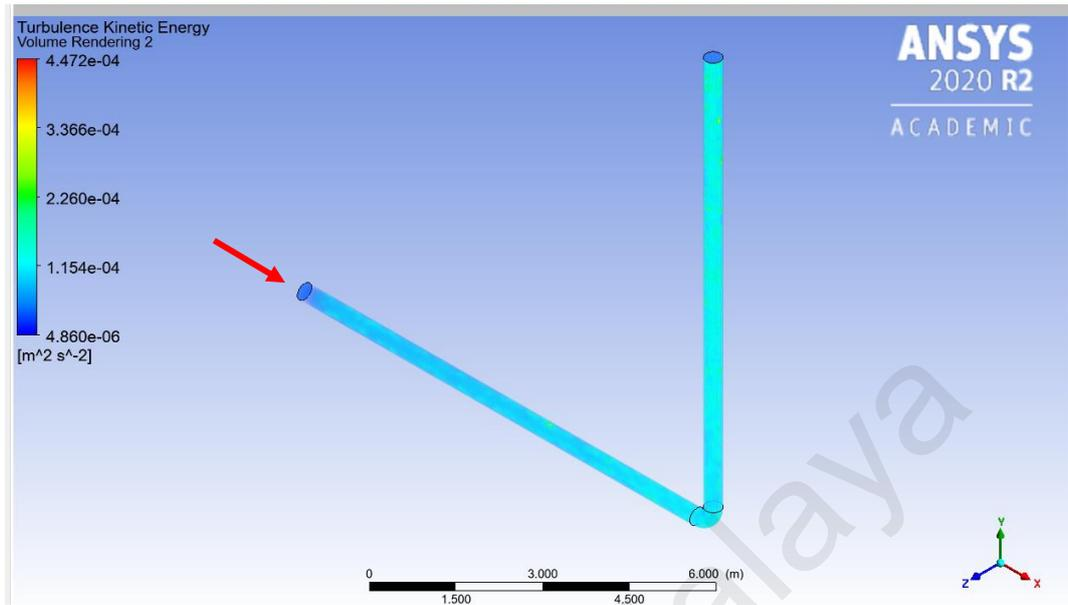
**Figure 4.9: Turbulence kinetic energy contour of 350 mm diameter pipe**
