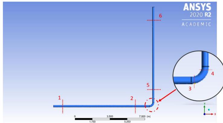
**Figure 3.3: Section on pipe for dynamic profile analysis**
