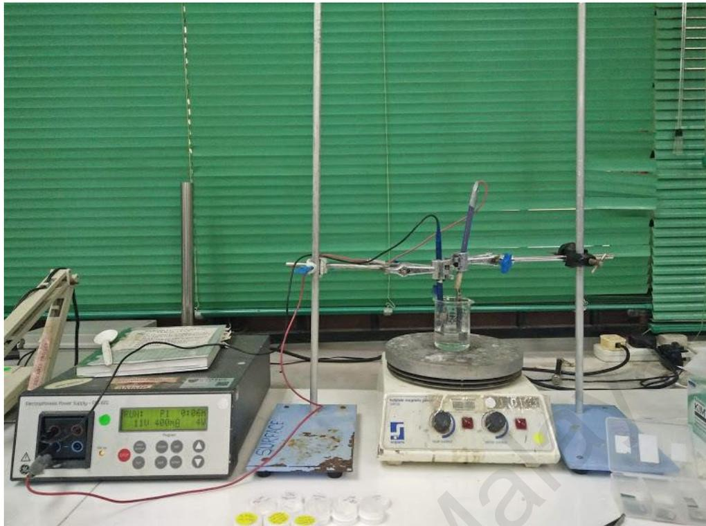
**Figure 3.4:** Experimental equipment to carry out anodization treatment process for producing aluminium oxide nano-porous arrays
