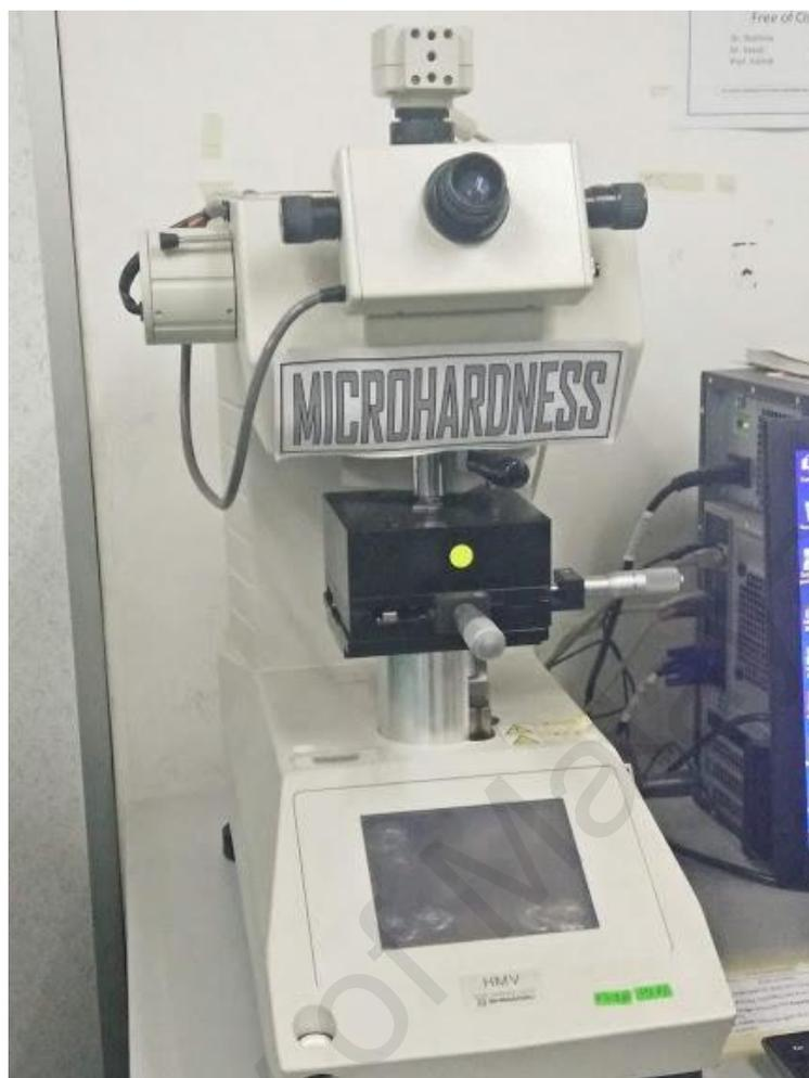
**Figure 3.8:** Vickers microhardness testing machine
