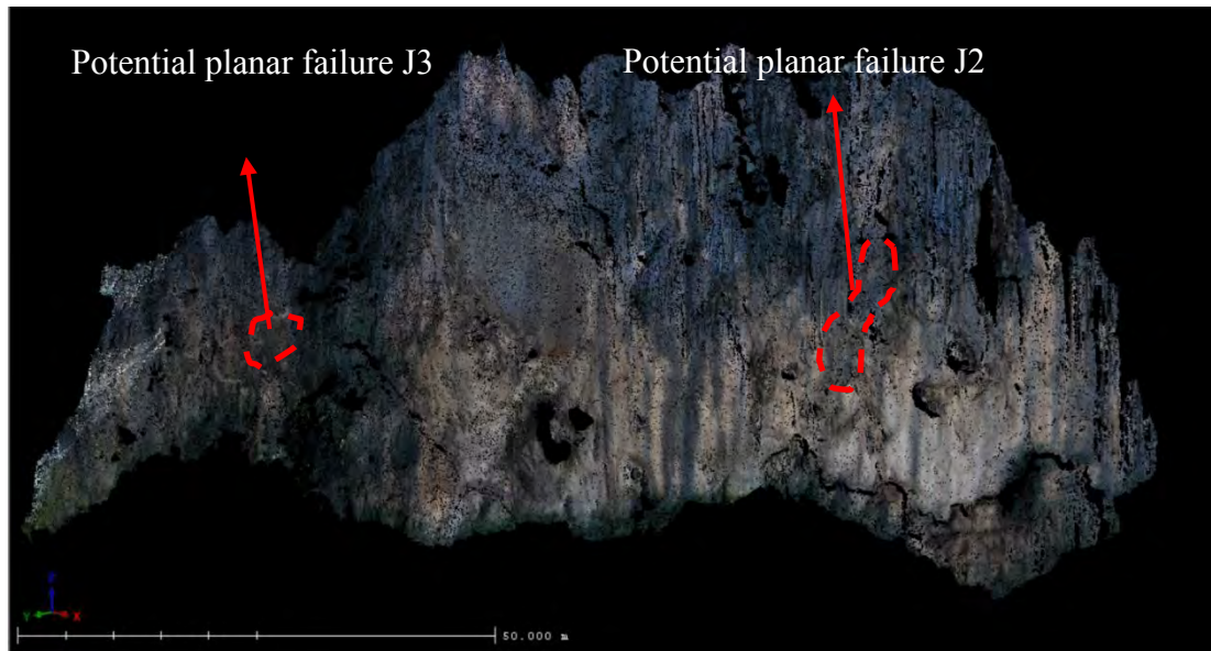
Figure 4.86: Overall view of Digital Terrain Model (DTM) of slope KYT (a) in true color display.
