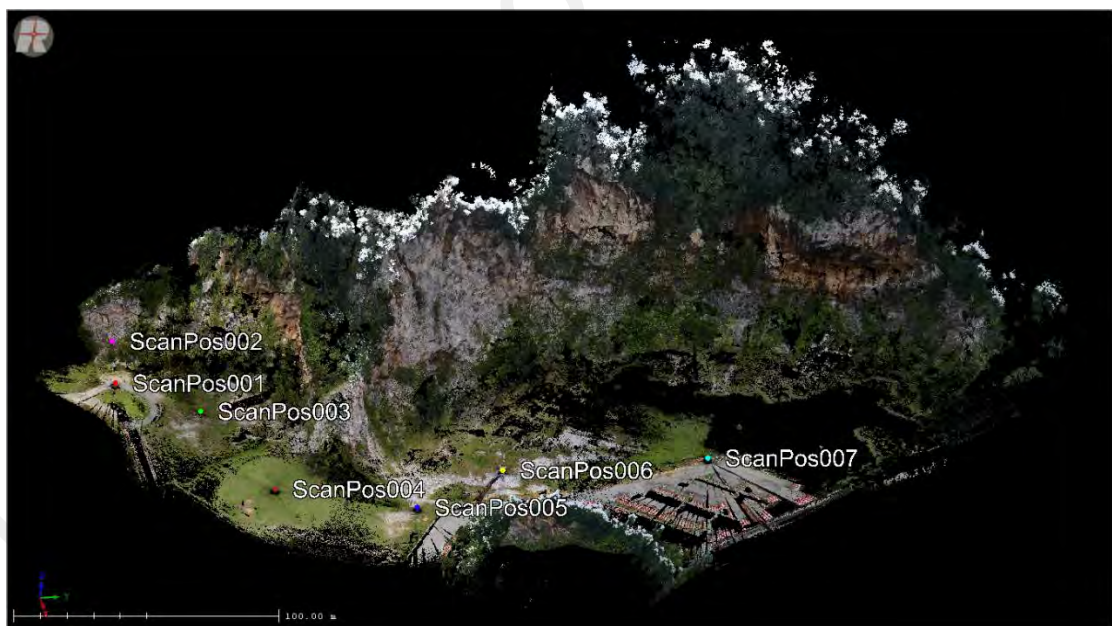
Figure 4.2: The position of 7 scanning position in the field, 3D model derived from RiScan Pro software.
