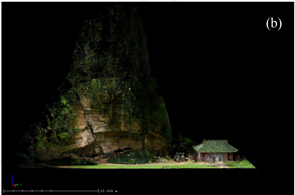
Figure 4.74: (a) Image taken by Nikon D800 camera showing the location of KLT 3 slope (b) Digital Terrain Model (DTM) of the slope with true color display.
