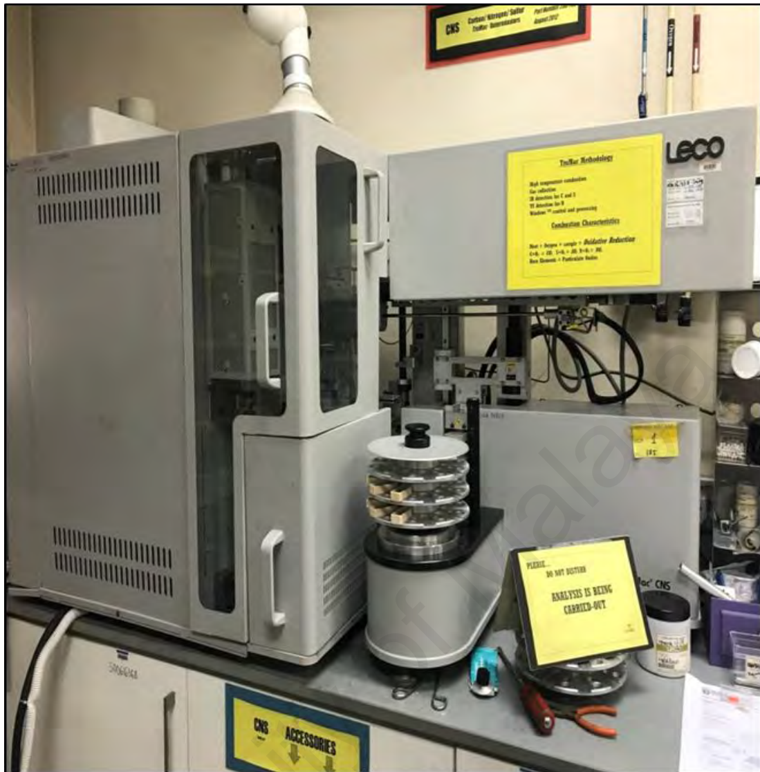
Figure 3.2: The CNS LECO TruMac analyzer used for soil TC analysis
