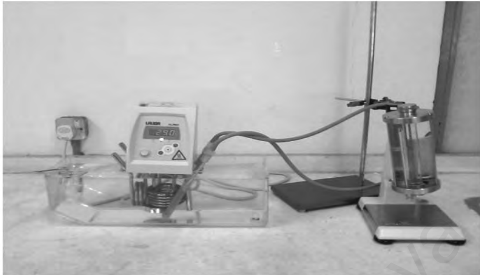
Figure 3.3: Falling ball viscometer setup. At the left-hand side is the unit pump connected to the thermostat and at the right-hand sight is gravitational tube filled with BBM.
