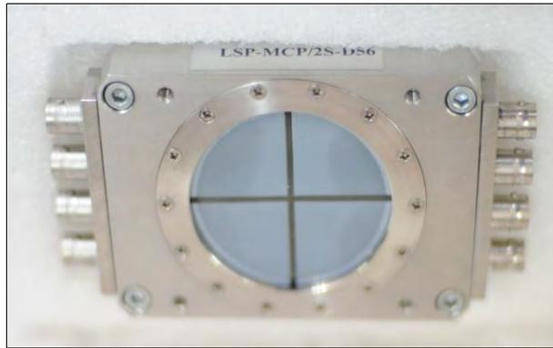
**Figure 3.17 (a):** Microchannel plate and pulse generator for MCP.
