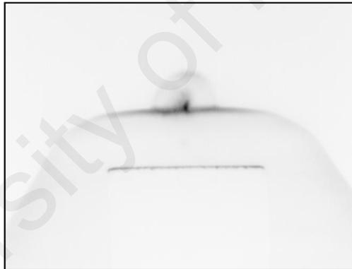
**Figure 4.3 (k):** First region pinch for induced shock wave move outward and form plasma bubble.
