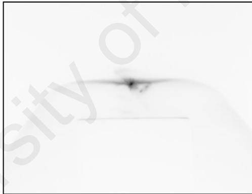
**Figure 4.3 (i):** First region pinch for the remaining plasma is compressed into another intense spot.
