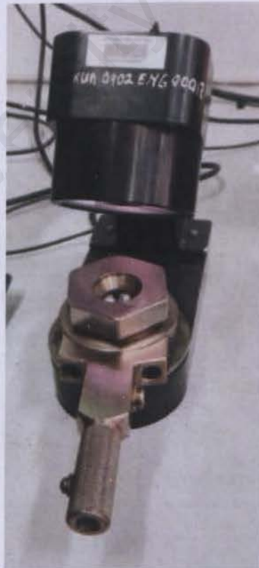
Figure 3.6: Optical microscope used to analyze the lower three ball bearings.
