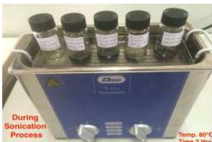
Figure 3.7: Stability and constancy of nanoparticles for two types of lubricant samples using a sonication device
