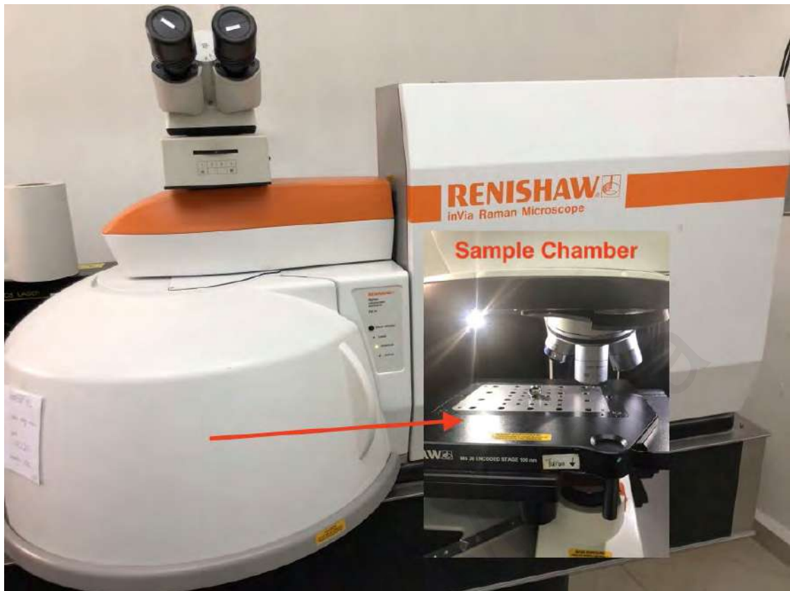
Figure 3.14: Raman microscope employed to investigate worn of scar balls
