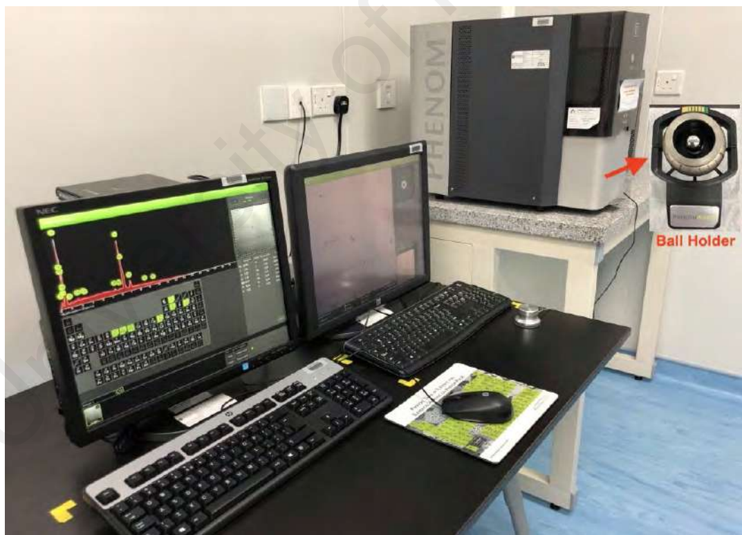
Figure 3.13: Energy-Dispersive X-ray Spectroscopy EDX/EDS and elemental mapping device with sample holder
