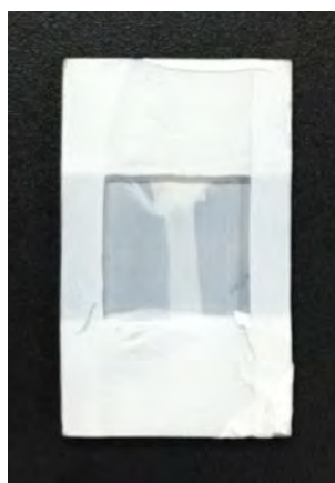
Figure 4.14 Sample masked with PTFE tape with square area exposed for ZnO coating.
