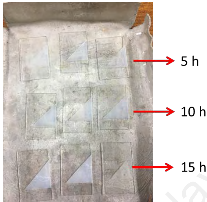
Figure 3.13 Successful ZnO nanorods coated glass substrates at growth time of 5 h, 10 h and 15 h.
